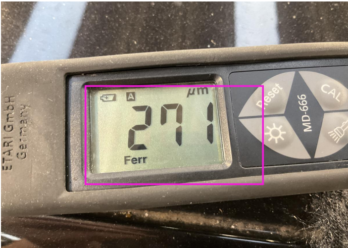
2. Door / Front Right Paint / Poor Previous Repair -
