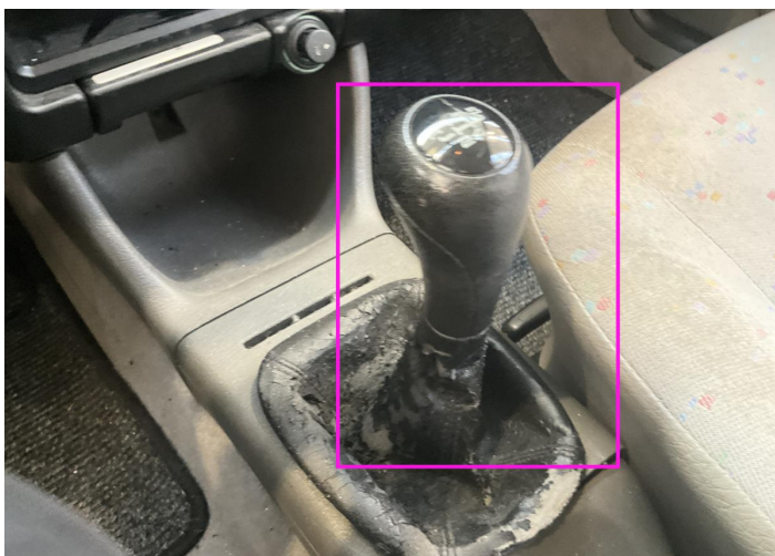
35. Gear Knob Interior / Broken -
