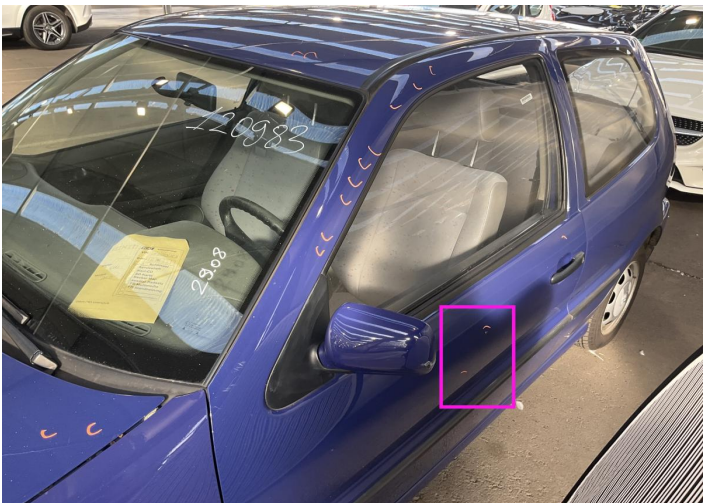
14. Door / Front Left Bodywork / Dent / Dent -
