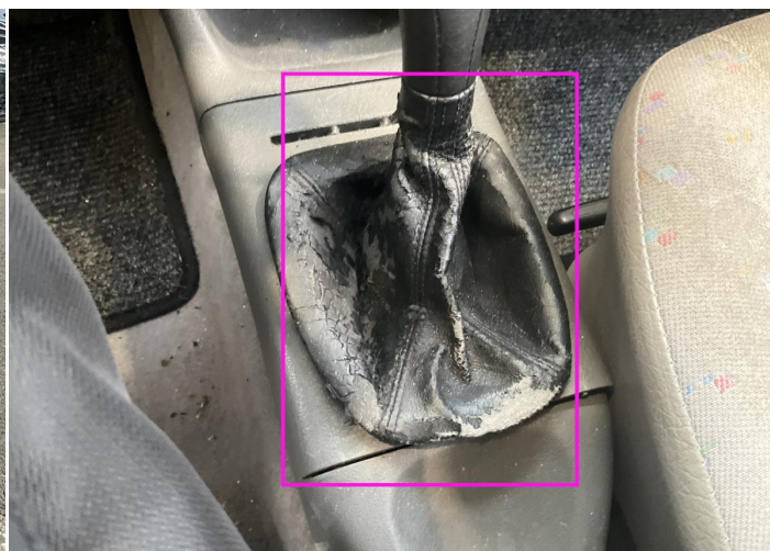
32. Gear Knob Interior / Worn - out -
