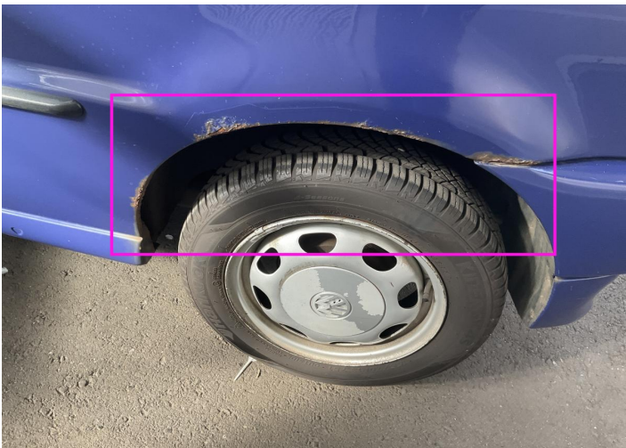
20. Fender / Back Left Paint / Corrosion -
