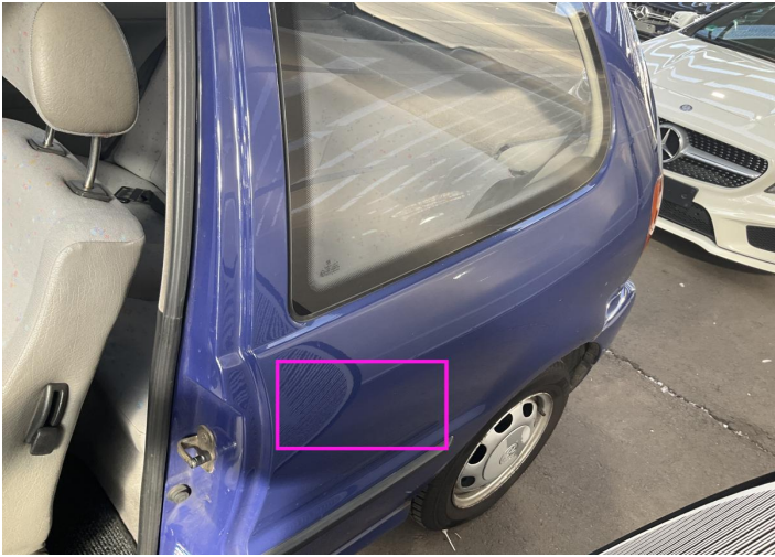
18. Fender / Back Left Bodywork / Dent / Dent -
