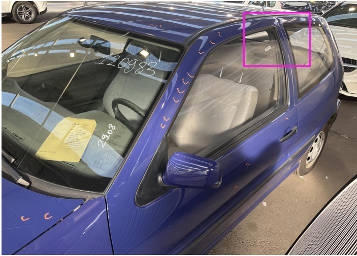
17. Door / Front Left Bodywork / Dent / Dent -
