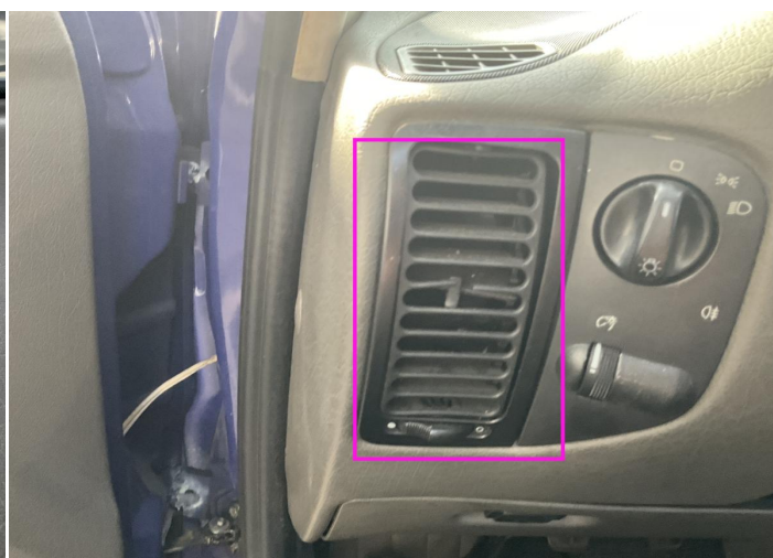
34. Aeration Grid / Front Left Interior / Broken -
