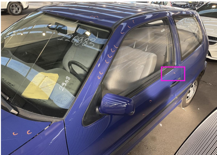
13. Door / Front Left Bodywork / Dent / Dent -
