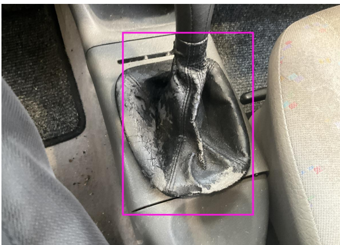
32. Gear Knob Interior / Worn - out -
