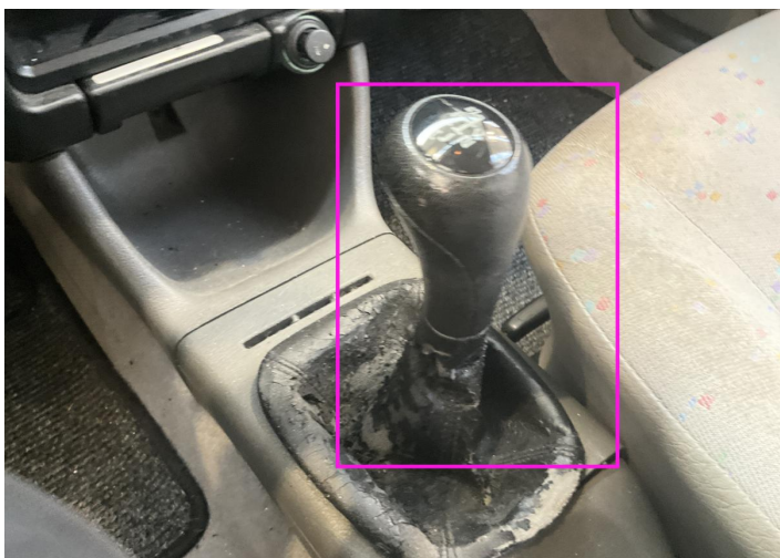
35. Gear Knob Interior / Broken -
