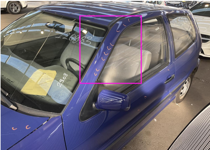
16. Door / Front Left Bodywork / Dent / Dent -
