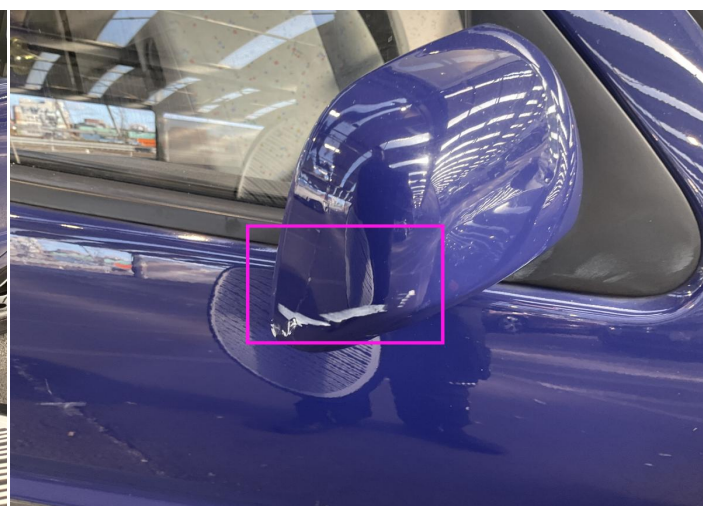
28. Mirror Repeater / Right Glass Break / Scratch / Scratch -
