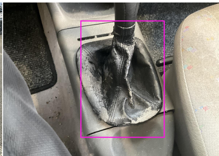
32. Gear Knob Interior / Worn - out -
