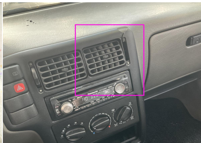
36. Aeration Grid / Front Center Interior / Broken -
