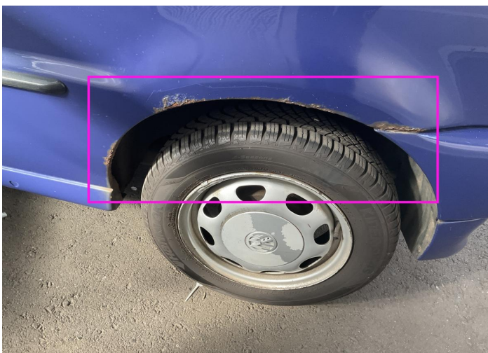
20. Fender / Back Left Paint / Corrosion -
