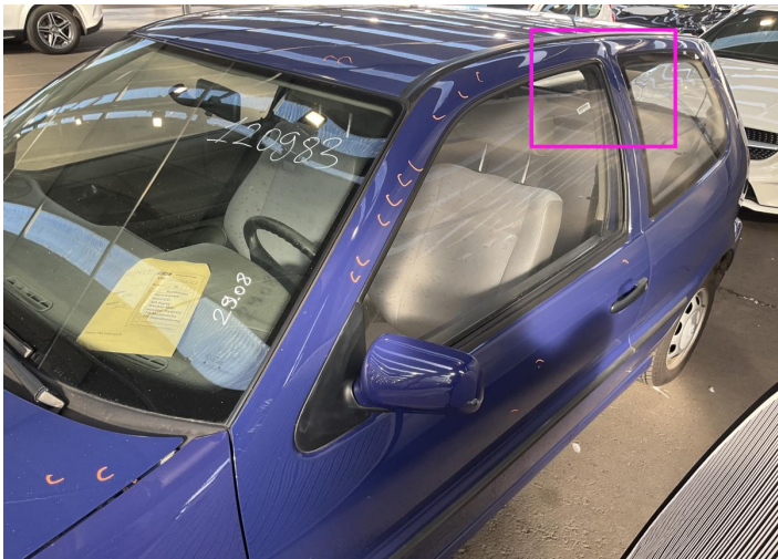
17. Door / Front Left Bodywork / Dent / Dent -
