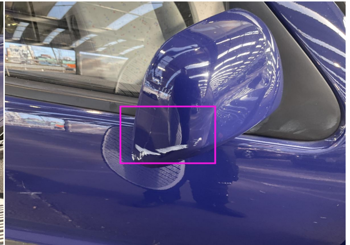
28. Mirror Repeater / Right Glass Break / Scratch / Scratch -
