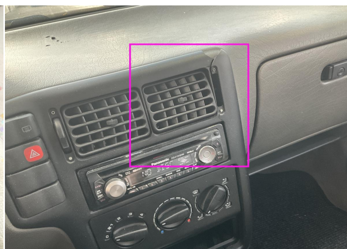
36. Aeration Grid / Front Center Interior / Broken -
