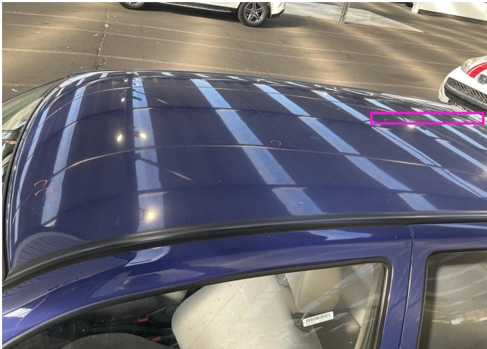
3. Roof Bodywork / Dent / Dent -
