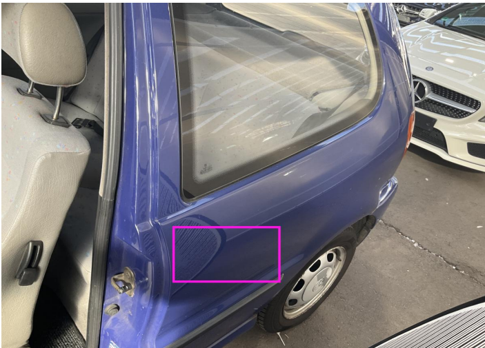
18. Fender / Back Left Bodywork / Dent / Dent -
