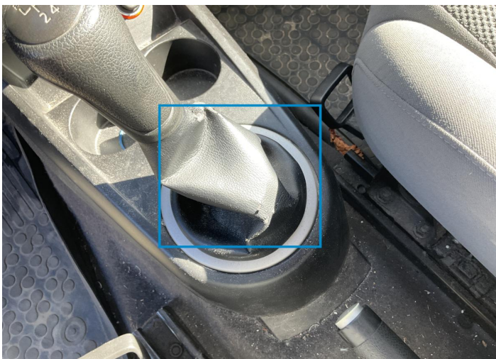
34. Gear Knob Interior / Ripped -
