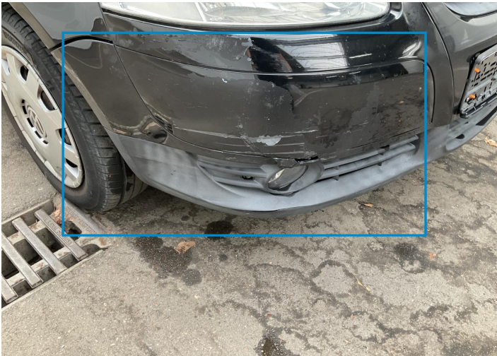
10. Bumper / Front Bodywork / Breakage / Crack -
