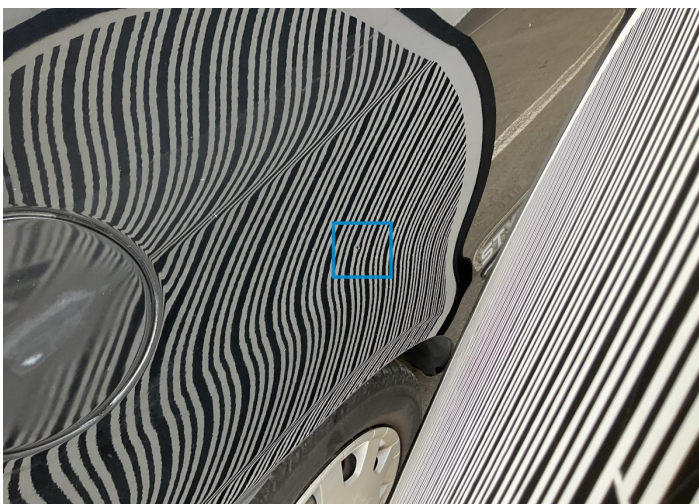
20. Side Panel / Back Right Bodywork / Dent / Dent -
