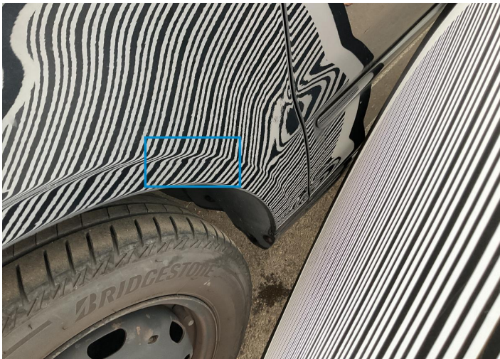
5. Fender / Front Left Bodywork / Dent / Dent -
