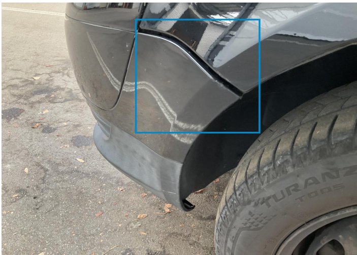
7. Bumper / Front Bodywork / Dent / Deformation -
