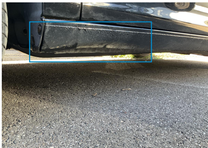
35. Rocker Panel / Center Left Bodywork / Dent / Dent -
