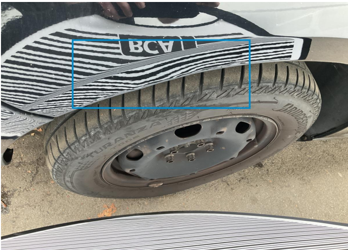
6. Fender / Front Left Bodywork / Dent / Dent -
