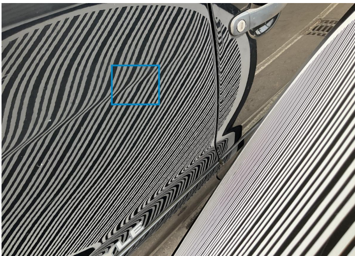
18. Side Panel / Back Right Bodywork / Dent / Dent -
