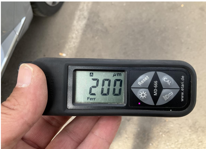
3. Door / Back Left Paint / Poor Previous Repair -
