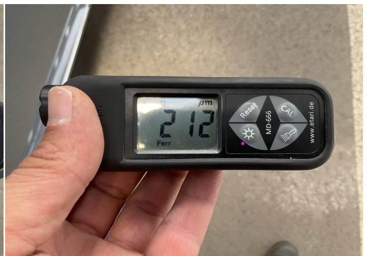
6. Door / Back Right Paint / Poor Previous Repair -
