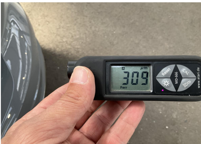
5. Tailgate Paint / Poor Previous Repair -
