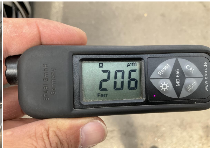
2. Roof Paint / Poor Previous Repair -
