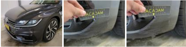
Bumper moulding FL, Scratch(es), Replace and paint
