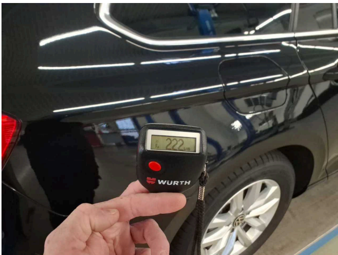
Side panel - rear right side: 222 µm
