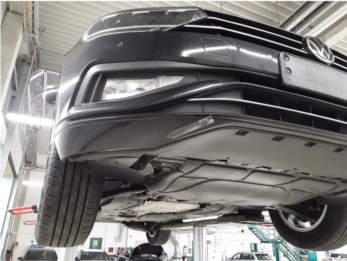
Damage 1: Front bumper: Bumper with Parktronic - Scratch(es) - Smart repair
