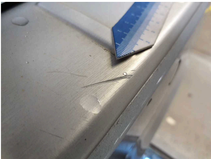
Wear and tear 6: Trim / covers: Boot sill cover - Scratched - No deduction
