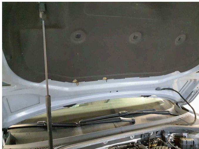
Damage 3: Bonnet: Insulation lining - Holes - Replace
