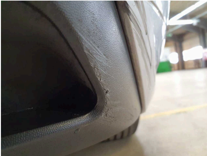
Damage 5: Rear bumper: Spoiler - Scratched - Replace
