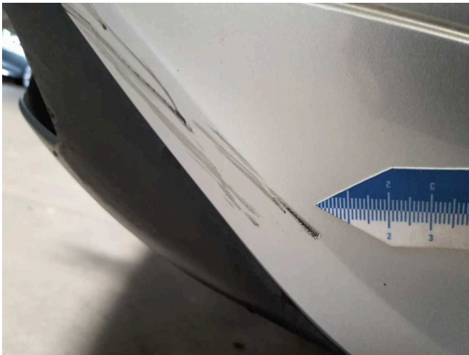
Damage 6: Rear bumper: Rear bumper - Scratched - Paint
