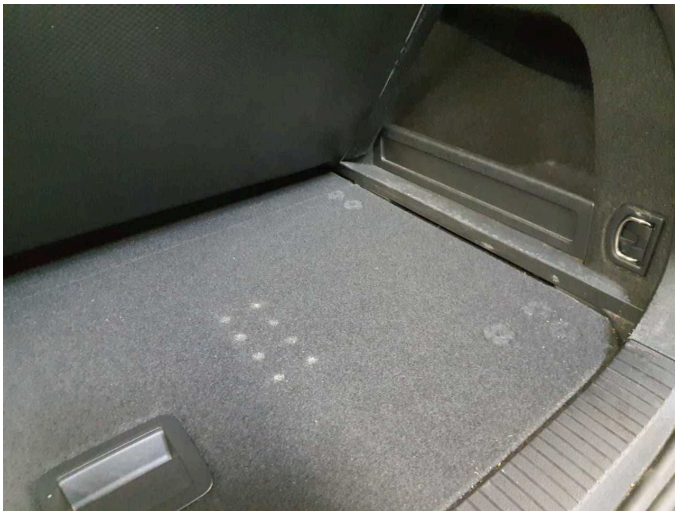
Wear and tear 1: Interior: Cargo area floor - Holes - No deduction
