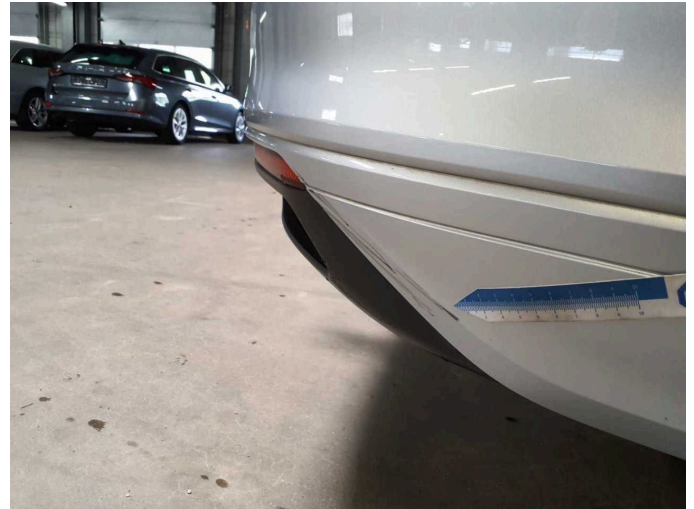
Damage 6: Rear bumper: Rear bumper - Scratched - Paint
