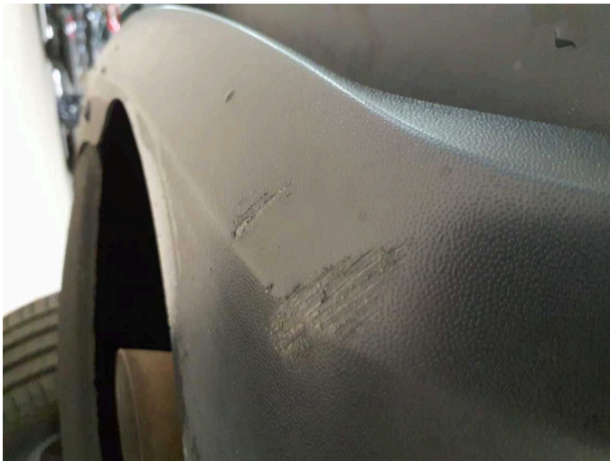
Damage 5: Rear bumper: Spoiler - Scratched - Replace
