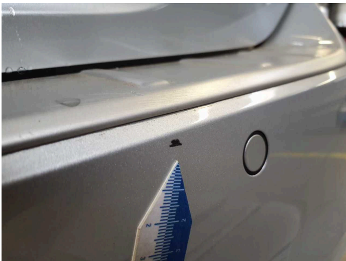
Damage 6: Rear bumper: Rear bumper - Scratched - Paint
