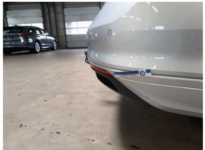
Damage 6: Rear bumper: Rear bumper - Scratched - Paint
