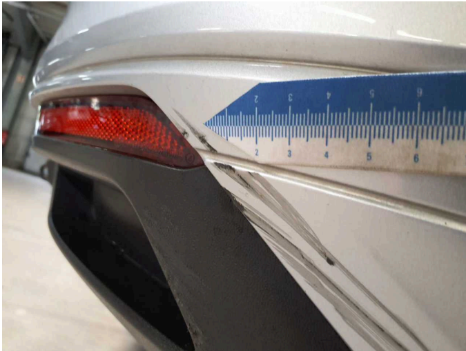
Damage 6: Rear bumper: Rear bumper - Scratched - Paint
