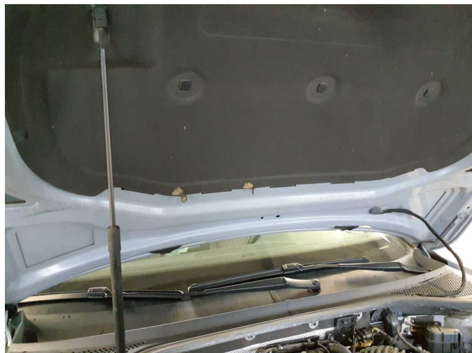
Damage 3: Bonnet: Insulation lining - Holes - Replace
