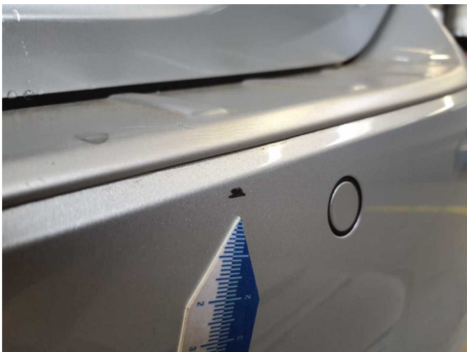
Damage 6: Rear bumper: Rear bumper - Scratched - Paint
