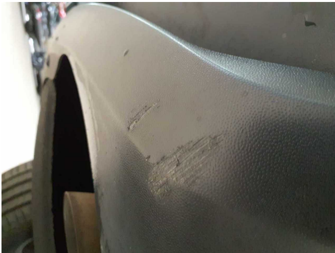
Damage 5: Rear bumper: Spoiler - Scratched - Replace
