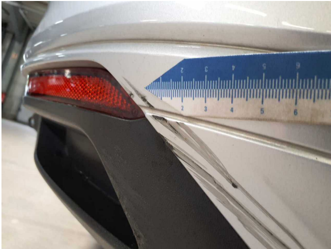
Damage 6: Rear bumper: Rear bumper - Scratched - Paint
