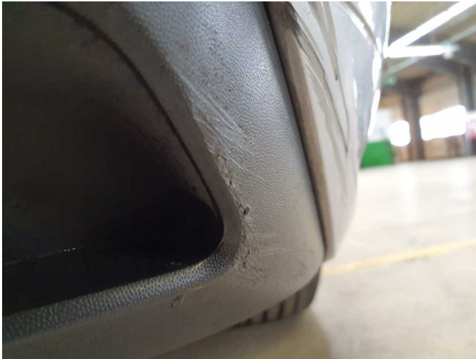
Damage 5: Rear bumper: Spoiler - Scratched - Replace
