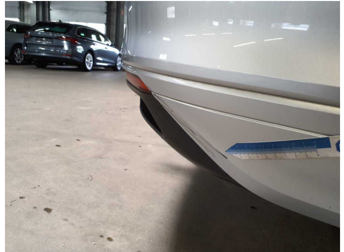
Damage 6: Rear bumper: Rear bumper - Scratched - Paint
