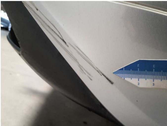
Damage 6: Rear bumper: Rear bumper - Scratched - Paint
