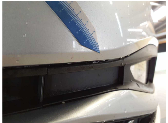
Damage 9: Front bumper: Front bumper (inkl. prüfen Lichtabdeckung) - Scratched - Repair and paint
