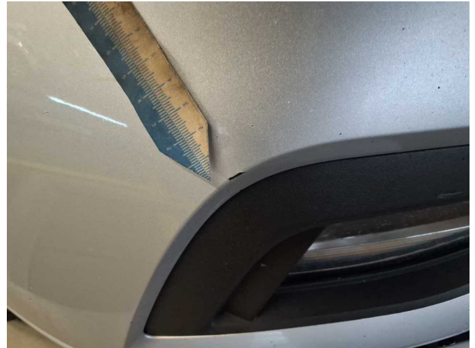
Damage 4: Front bumper: Front bumper - Scratched - Paint
