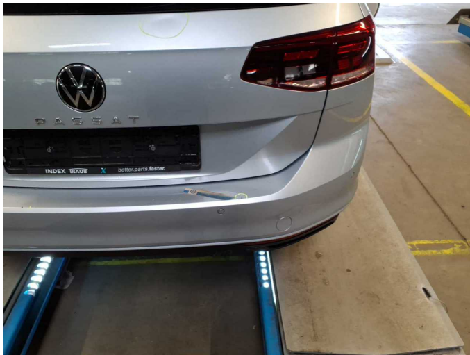
Damage 5: Rear bumper: Rear bumper - Scratch(es) - Paint
