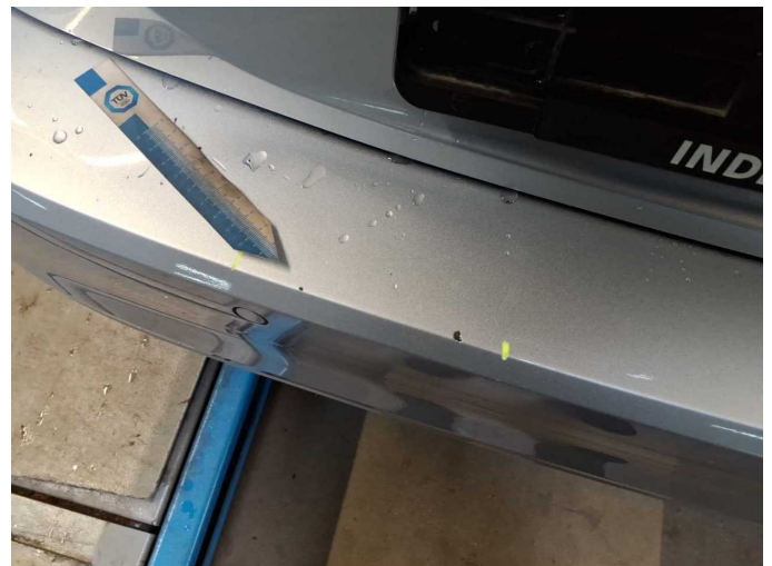
Damage 5: Rear bumper: Rear bumper - Scratch(es) - Paint
