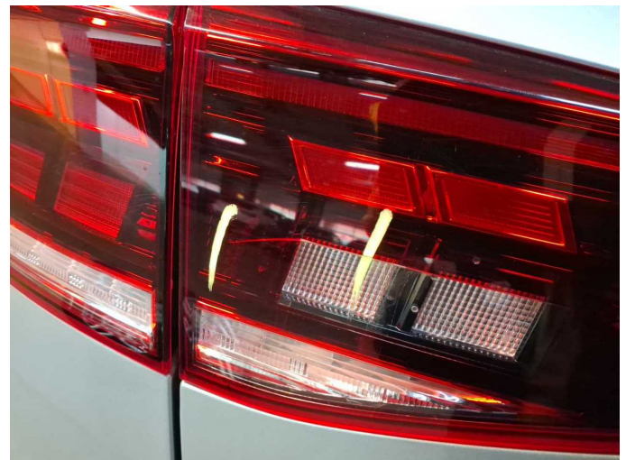
Damage 3: Tail light: Tail lamp - left side - Broken / torn - Replace
