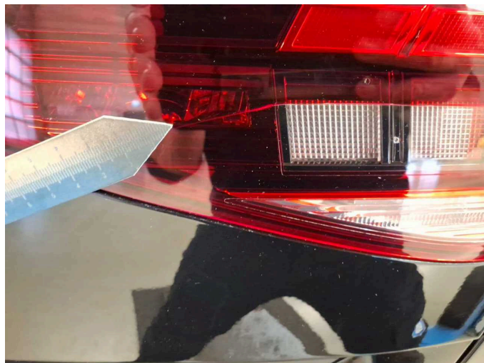
Damage 6: Tail light: Tail lamp - right side (innen) - Broken / torn - Replace
