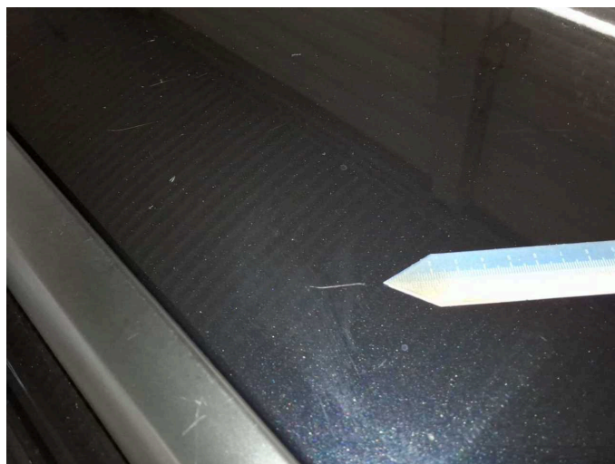
Damage 8: Roof: Roof - Scratch(es) - Paint
