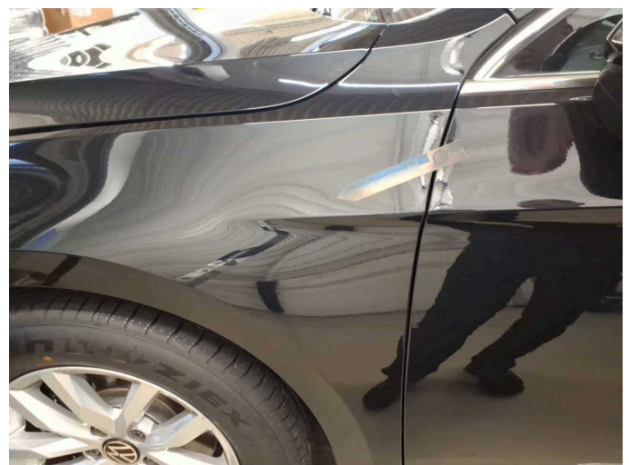
Damage 3: Mudguard - left side: Mudguard - left side - Scratch(es) - Smart repair
