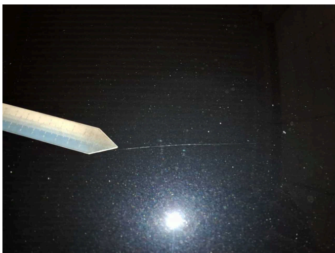
Damage 7: Bonnet: Bonnet (+ Steinschläge) - Scratch(es) - Paint
