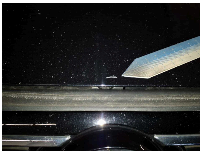
Damage 7: Bonnet: Bonnet (+ Steinschläge) - Scratch(es) - Paint
