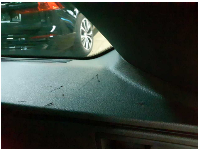
Damage 8: Trim / covers: Cargo area - lining - right side - Scratched - Replace
