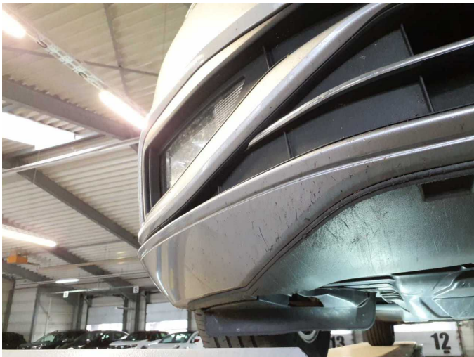
Damage 10: Front bumper: Front bumper (Sandstrahleffekt) - Stone chips - Paint
