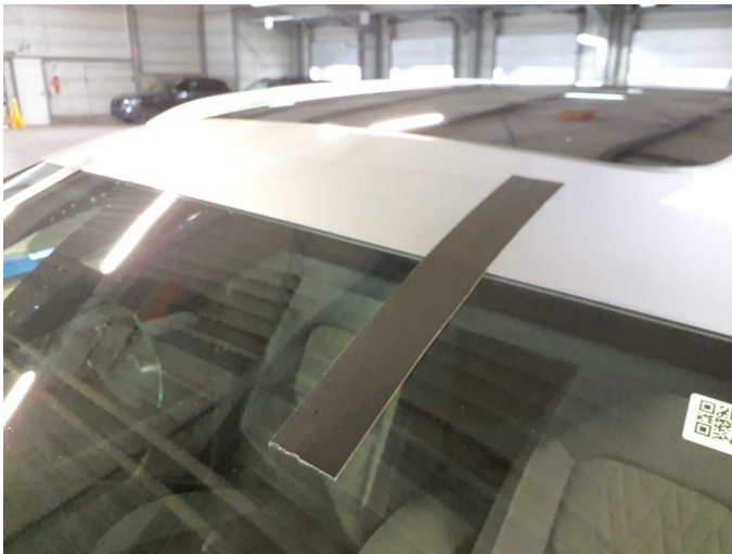
Damage 1: Body: Body - Glued / labelled - De-glue / neutralise
