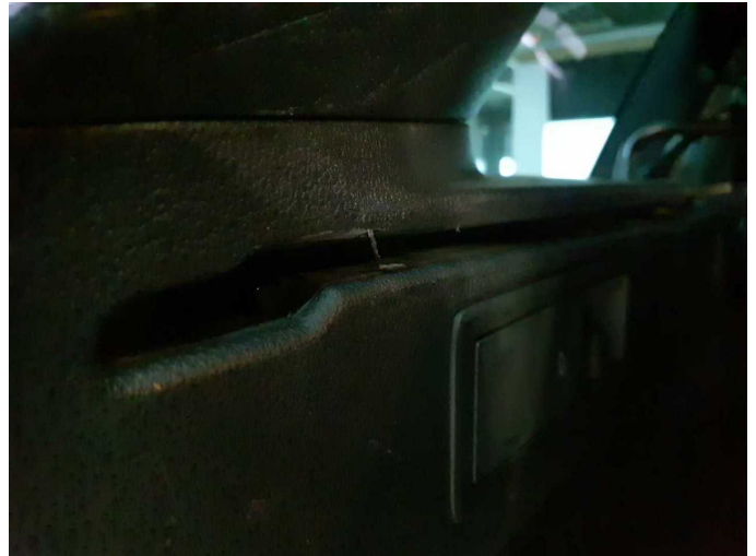
Damage 9: Trim / covers: Cargo area - lining -left side - Scratched - Replace
