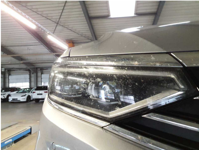
Wear and tear 7: Headlight: Headlight - right side (+verschmutzt) - Stone chips - No deduction
