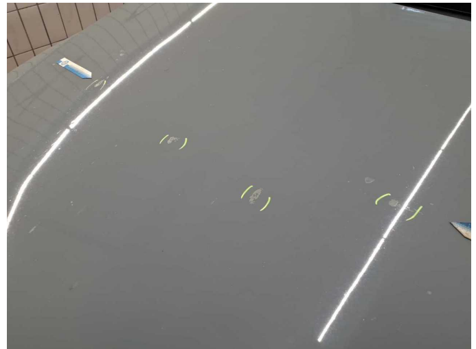
Damage 11: Bonnet: Bonnet (+ Harz entfernen) - Dent / paintcoat damage - Repair and paint
