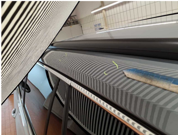
Damage 6: Roof: Roof rail - left side - dent(s) - Smart repair
