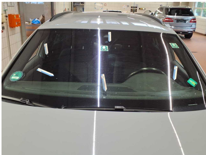
Damage 12: Vehicle glazing: Windscreen - Stone chips - Replace
