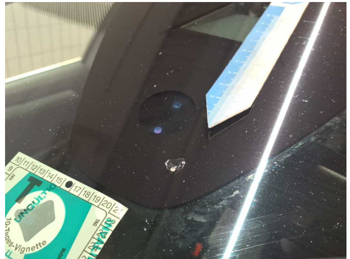
Damage 12: Vehicle glazing: Windscreen - Stone chips - Replace
