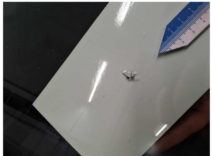
Damage 12: Vehicle glazing: Windscreen - Stone chips - Replace
