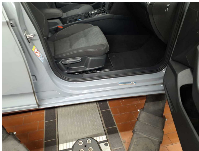
Damage 5: Sill - right side: Sill - dent(s) - Smart repair
