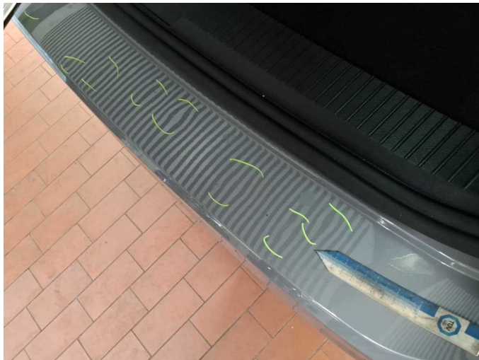
Damage 9: Rear bumper: Rear bumper - Deformed - Repair and paint
