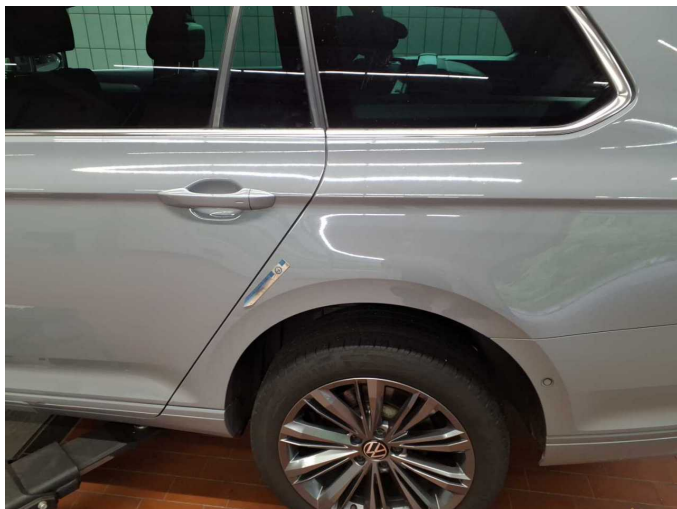
Damage 8: Side panel - rear left side: Side panel (An Kante) - dent(s) - Repair and paint
