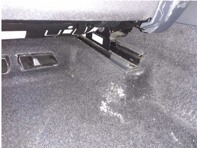
Damage 8: Interior: Interior (Schimmelbildung) - Soiled - Clean
