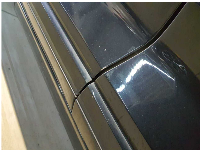
Wear and tear 10: Door - front left side: Door edge - Scratched - Smart repair
