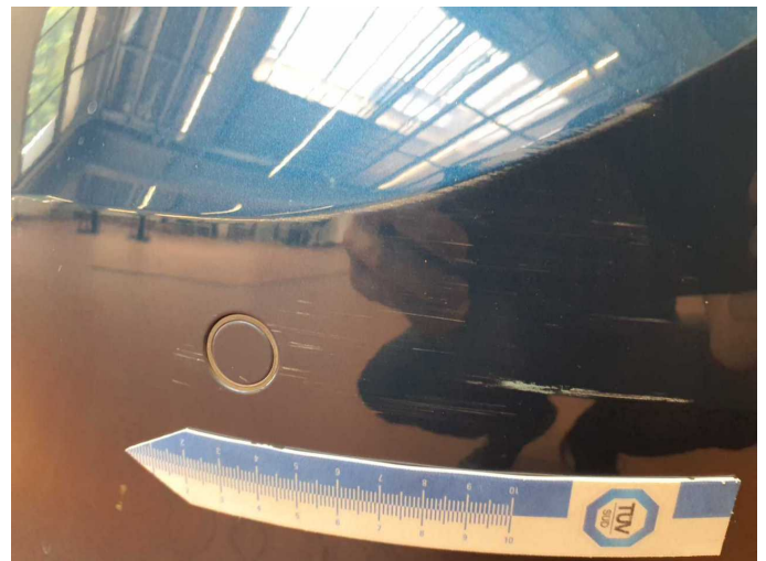
Damage 9: Rear bumper: Rear bumper - Scratched - Paint
