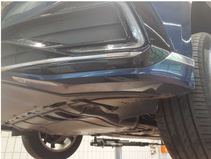
Damage 7: Front bumper: Spoiler - Scratched - Paint
