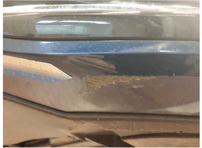
Damage 7: Front bumper: Spoiler - Scratched - Paint
