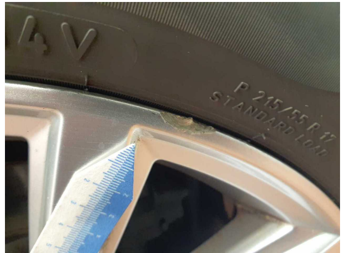
Damage 8: Wheel / tyres: Alloy rim - front right side - Damaged - Replace
