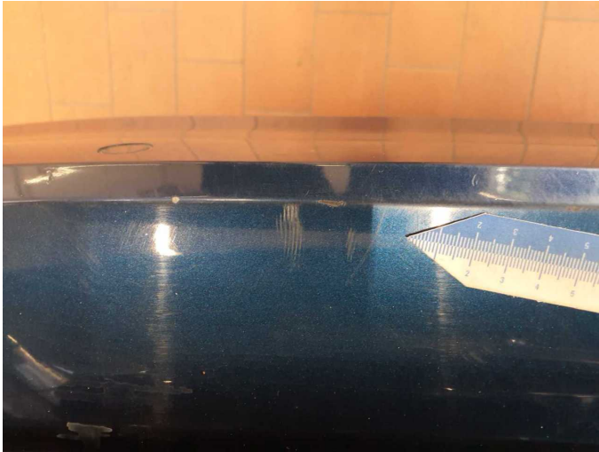
Damage 9: Rear bumper: Rear bumper - Scratched - Paint
