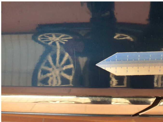
Damage 6: Door - rear left side: Door - Scratch(es) - Smart repair
