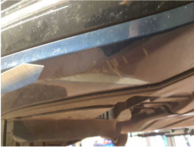
Damage 7: Front bumper: Spoiler - Scratched - Paint
