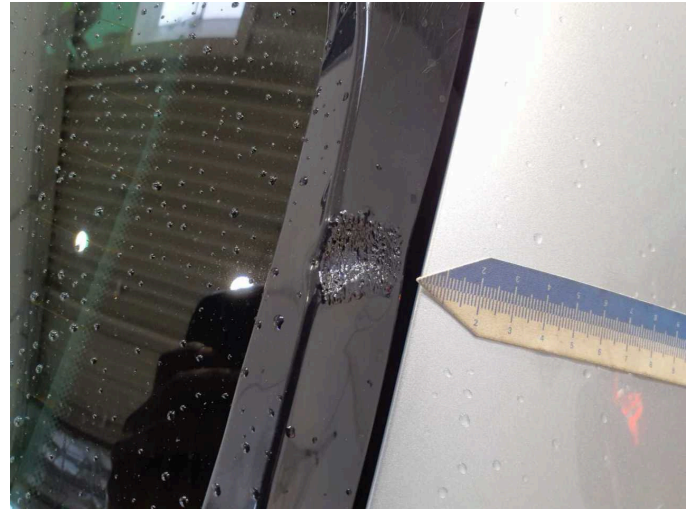
Damage 2: Boot lid / rear door: Rear spoiler (rechts) - Damaged - Replace
