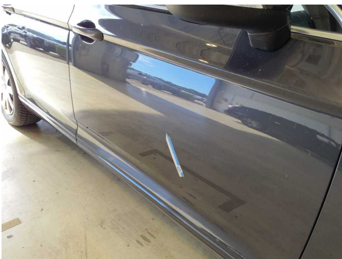
Damage 2: Door - front right side: Door - dent(s) - Smart repair
