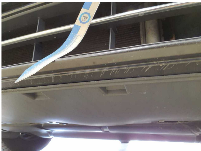
Damage 4: Front bumper: Front bumper - Scratch(es) - Paint
