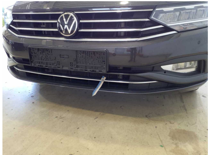
Damage 4: Front bumper: Front bumper - Scratch(es) - Paint
