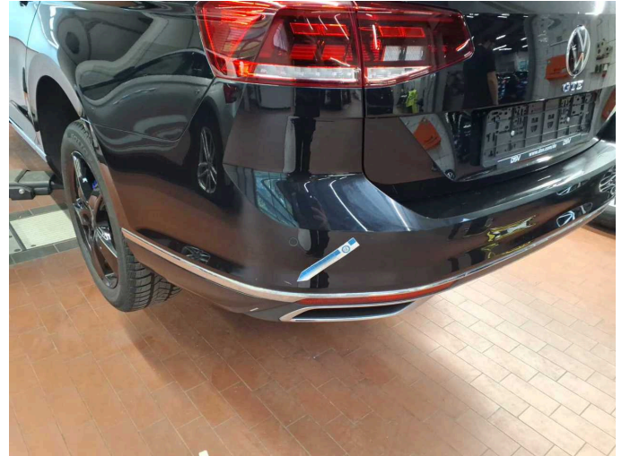
Damage 4: Rear bumper: Rear bumper - Scratch(es) - Paint
