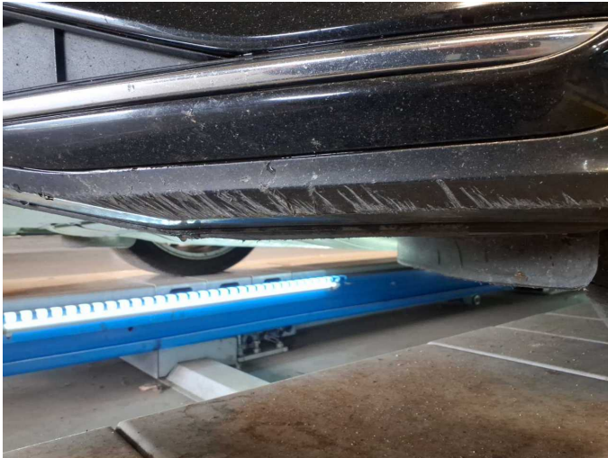
Damage 11: Front bumper: Spoiler - Scratched - Paint
