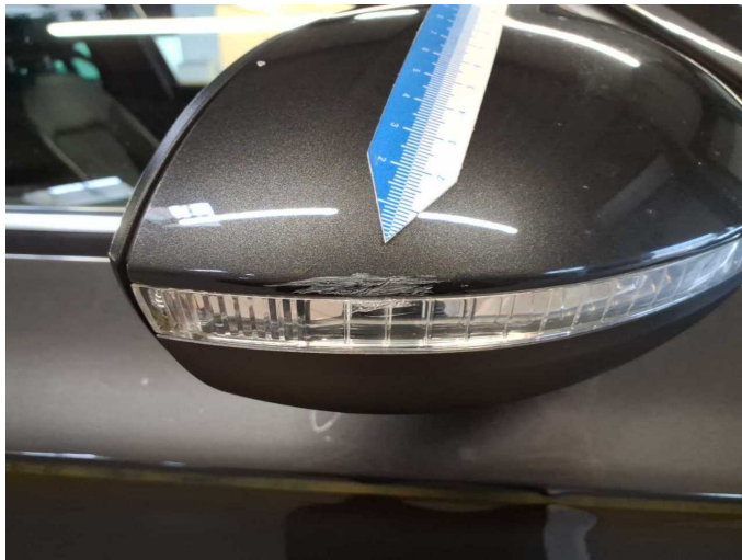
Damage 6: Wing mirror - right side: Cap - Scratched - Paint
