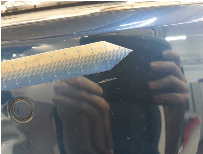
Wear and tear 6: Front bumper: Front bumper - Scratch(es) - No deduction
