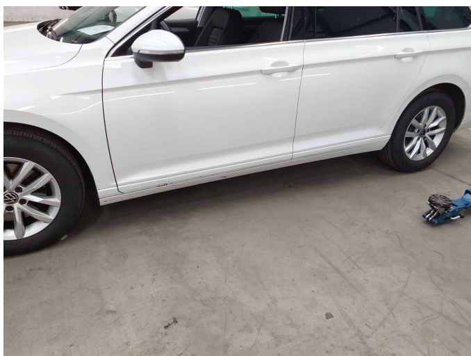
Damage 4: Body: Body (linke Fahrzeugseite) - Scratched - Repair and paint
