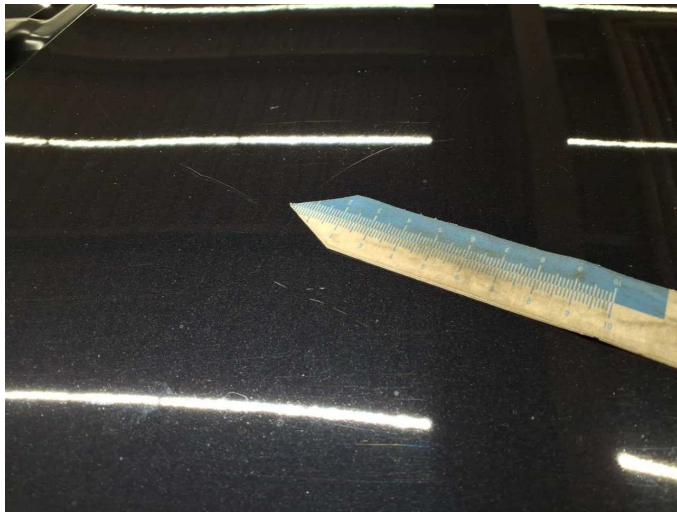
Damage 16: Bonnet: Bonnet - Scratch(es) - Paint
