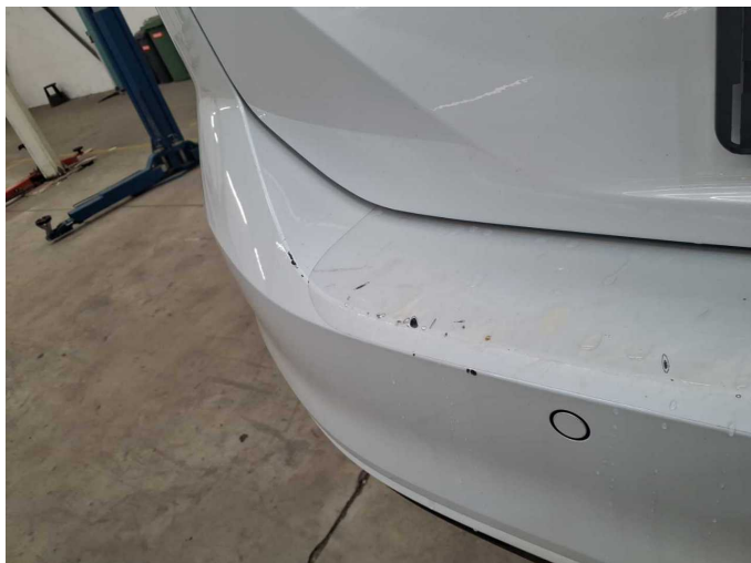
Damage 5: Rear bumper: Rear bumper - Scratched - Paint
