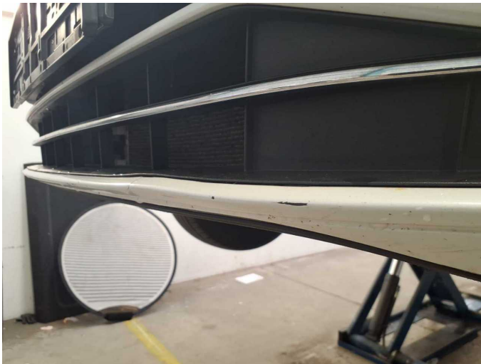
Damage 4: Front bumper: Front bumper - Scratched - Paint
