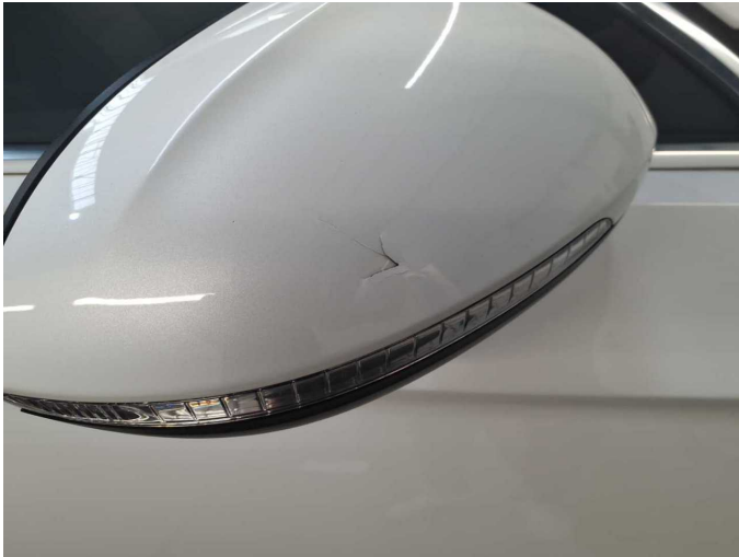
Damage 3: Wing mirror - right side: Cap - Broken / torn - Replace
