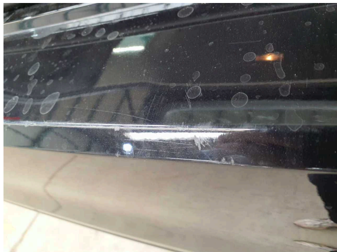
Damage 5: Rear bumper: Rear bumper - Scratched - Paint
