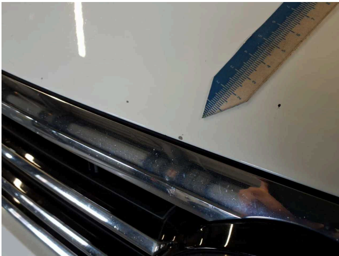
Damage 11: Bonnet: Bonnet (Steinschlag) - Deformed - Repair and paint
