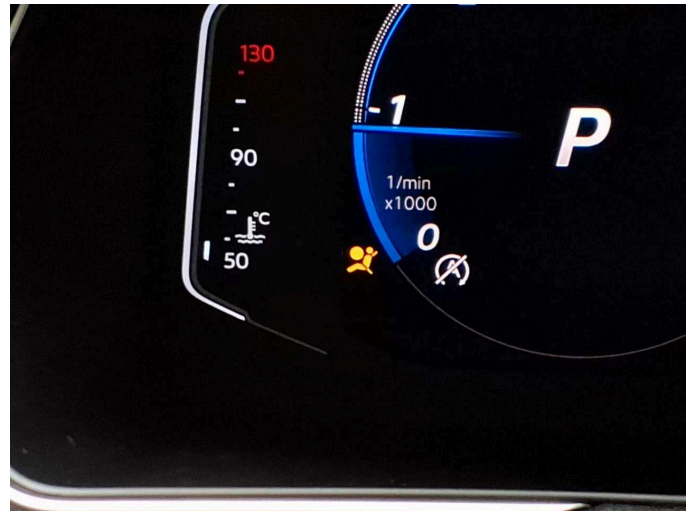
Damage 7: Airbag systems: Airbag system (Airbag Lampe an) - Functional / admissibility - Perform diagnosis
