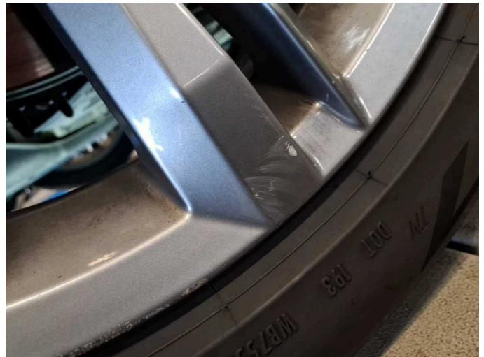
Damage 9: Wheel / tyres: Alloy rim - front left side (Materialabtrag) - Scratched - Replace
