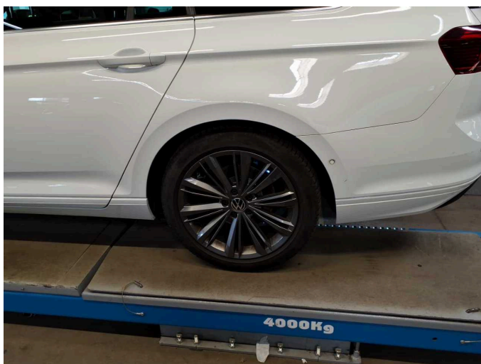
Damage 8: Wheel / tyres: Alloy rim - rear left side (Materialabtrag) - Scratched - Replace
