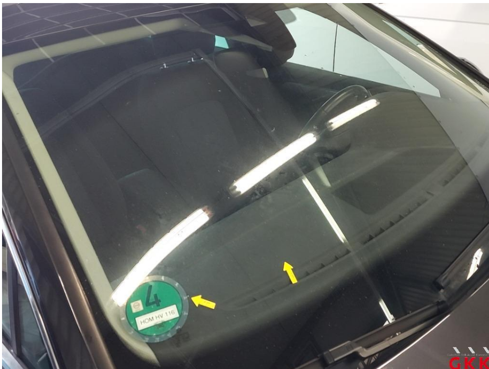
Picture 29 front screen, with rain sensor and frontcamera, chipping with cracking
