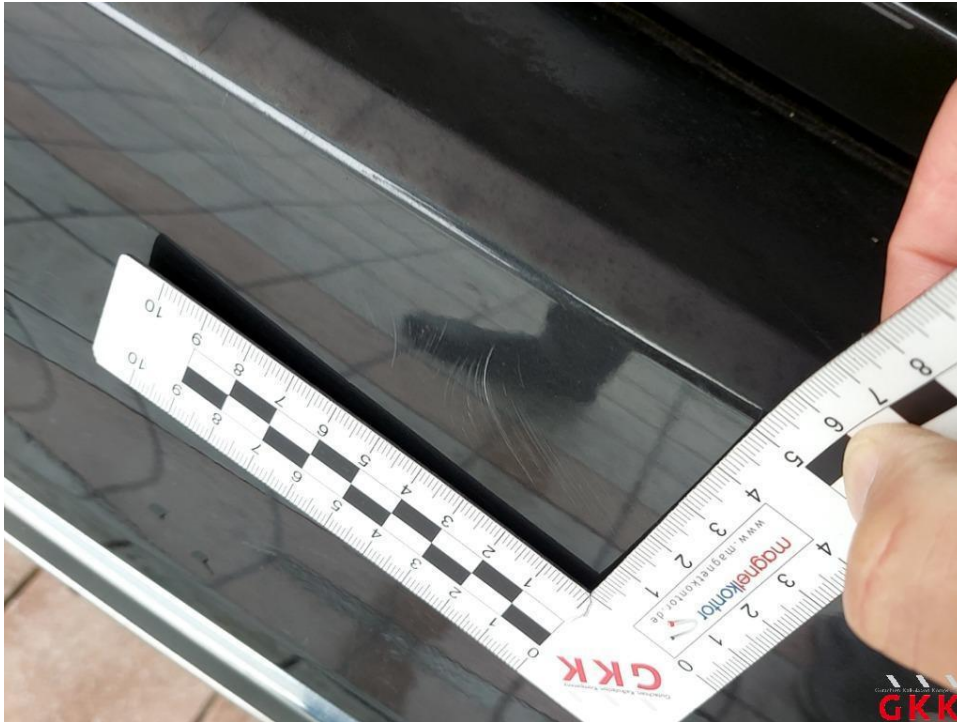
Picture 34 bumper rear, panel -painted-, scratched
