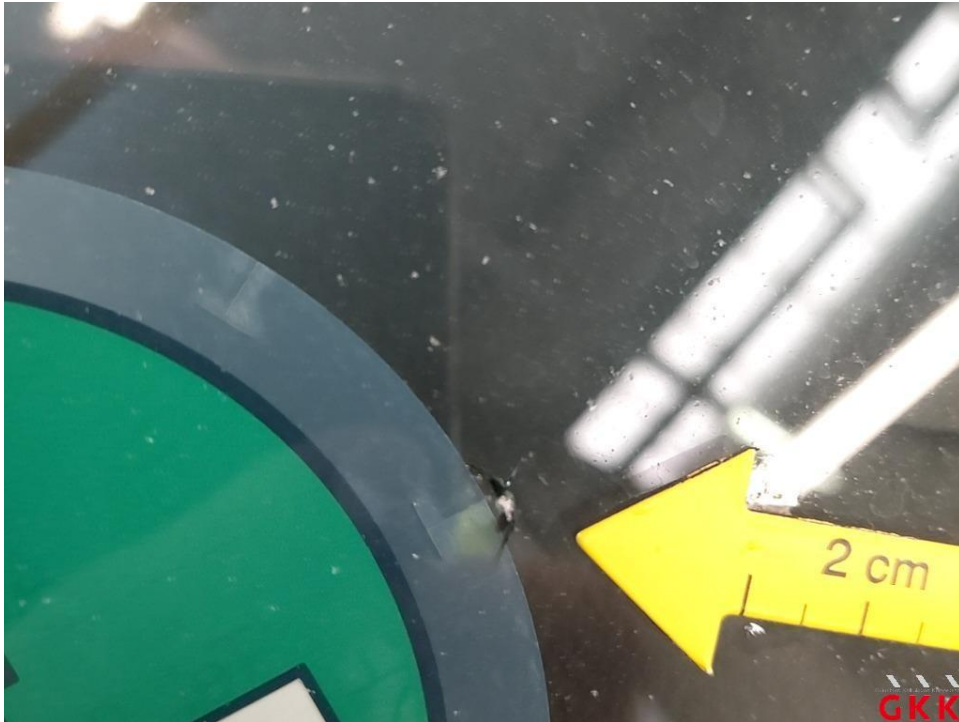
Picture 30 front screen, with rain sensor and frontcamera, chipping with cracking
