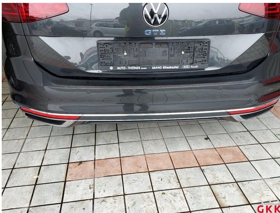
Picture 33 bumper rear, panel -painted-, scratched
