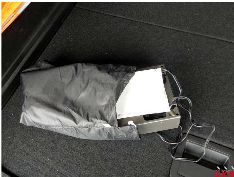
Picture 39 tyre repair set, refill bottle, missing
