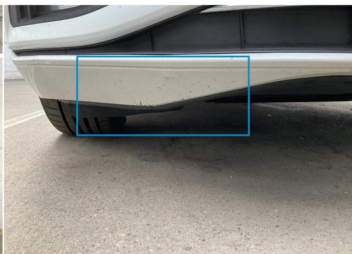
4. Bumper / Front Paint / Scratch / Scuff -
