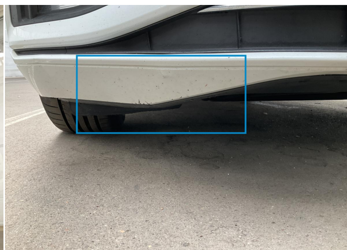
4. Bumper / Front Paint / Scratch / Scuff -
