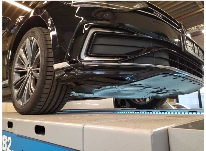
Damage 13: Front bumper: Front bumper (inkl. Spoiler, Radhausabd. unten vorne) - Deformed - repair according to calculation
