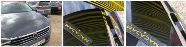
Bumper F, Scratch(es), Repair and paint (complete)
