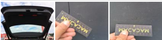
Internal boot lining R, Hole, Smart repair
