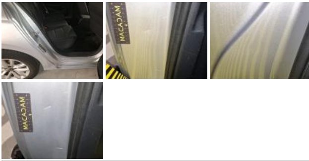
Step R, Dent(s) and scratch(es), Acceptable
