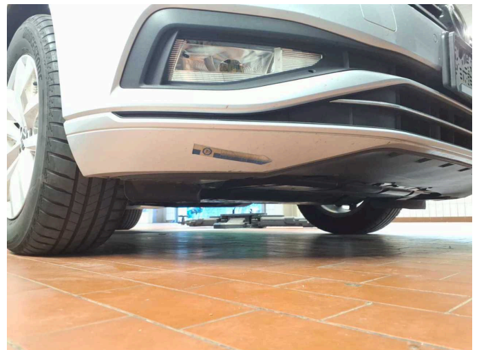
Damage 5: Front bumper: Spoiler - Scratched - Paint
