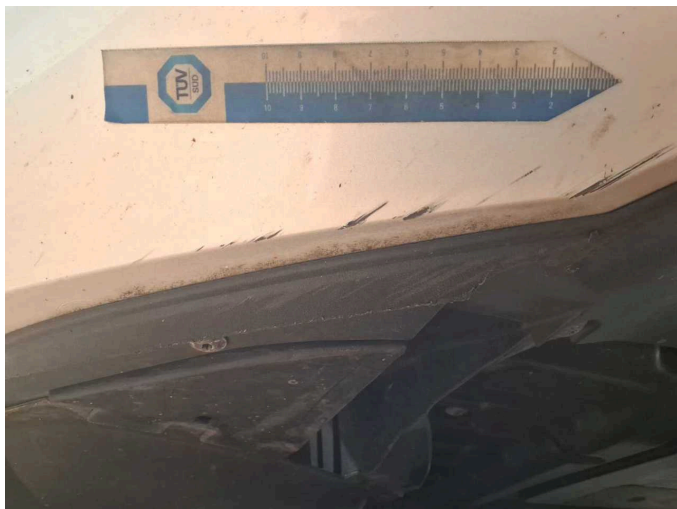
Damage 5: Front bumper: Spoiler - Scratched - Paint
