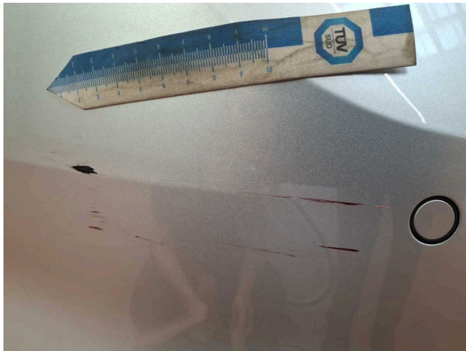
Damage 7: Rear bumper: Rear bumper - Scratched - Paint
