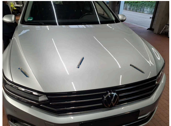
Damage 8: Bonnet: Bonnet - Stone chips - Paint
