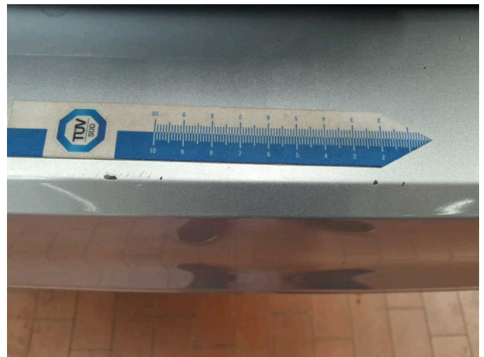
Damage 7: Rear bumper: Rear bumper - Scratched - Paint
