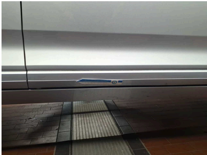
Damage 2: Door - front right side: Brightware - lower - Scratch(es) - Smart repair
