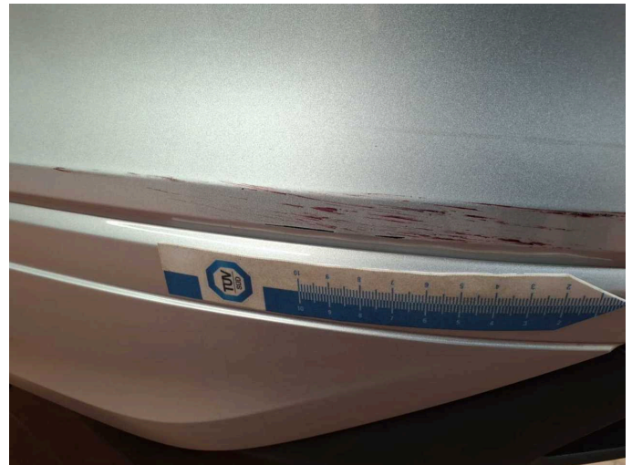
Damage 7: Rear bumper: Rear bumper - Scratched - Paint
