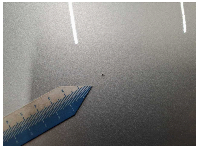
Damage 8: Bonnet: Bonnet - Stone chips - Paint
