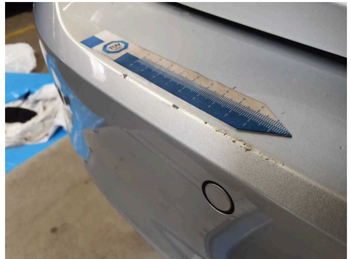
Damage 4: Rear bumper: Rear bumper - Scratched - Paint
