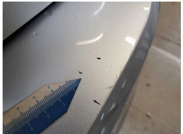
Damage 4: Rear bumper: Rear bumper - Scratched - Paint
