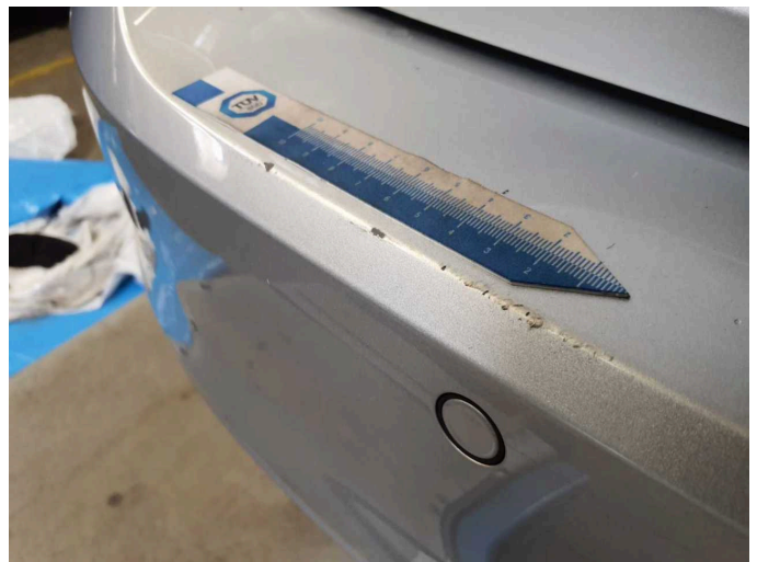
Damage 4: Rear bumper: Rear bumper - Scratched - Paint
