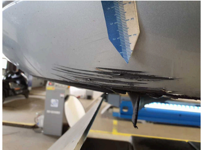
Damage 5: Front bumper: Front bumper (Steinschlag) - Scratched - Repair and paint
