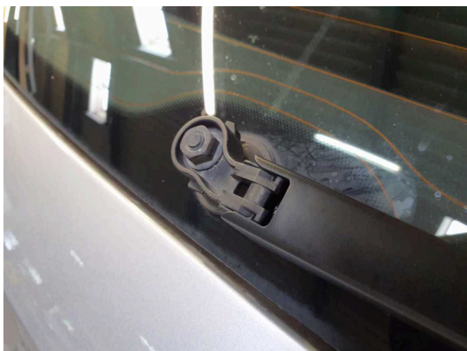
Damage 2: Screen cleaning: Wiper arm - rear (Abdeckung) - Missing - Replace
