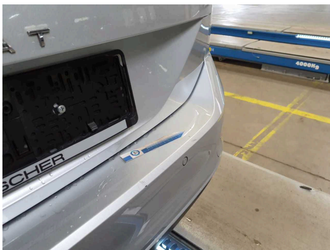
Damage 4: Rear bumper: Rear bumper - Scratched - Paint
