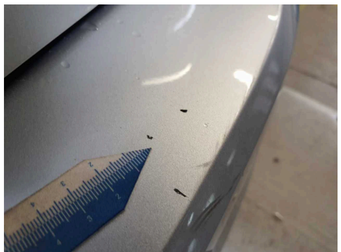
Damage 4: Rear bumper: Rear bumper - Scratched - Paint
