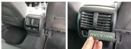
Backrest cover RL, Damaged, Smart repair
