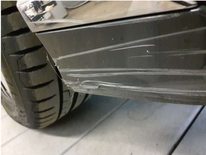
Damage 11: Front bumper: Spoiler (Materialabtrag) - Scratched - Replace
