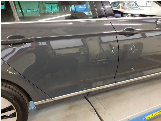
Damage 14: Door - rear right side: Door - dent(s) - Repair and paint
