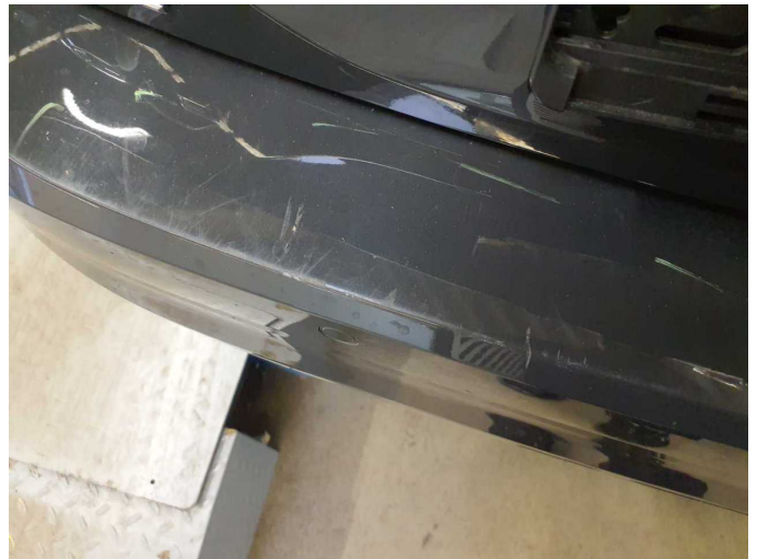
Damage 13: Rear bumper: Rear bumper - Scratched - Paint
