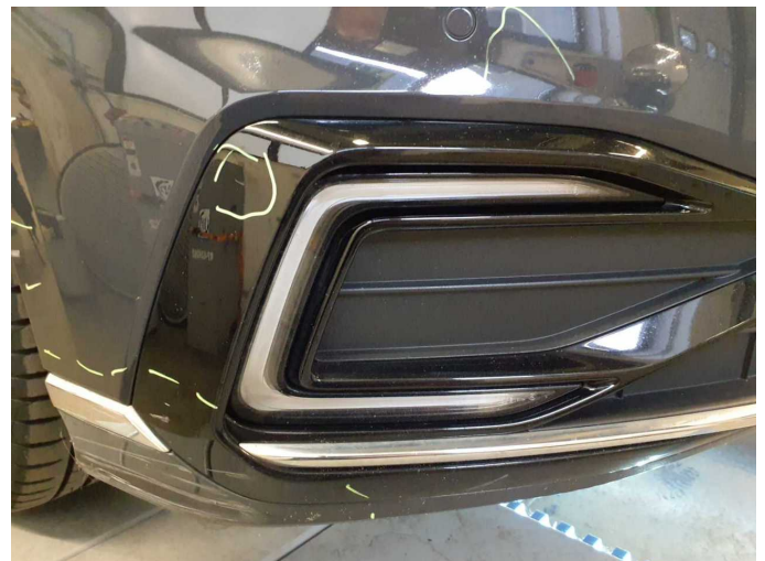
Damage 5: Front bumper: Cover bumper - front (Materialabtrag) - Scratched - Replace
