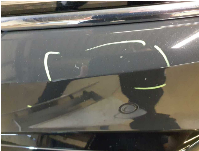
Damage 12: Front bumper: Front bumper - Scratched - Paint
