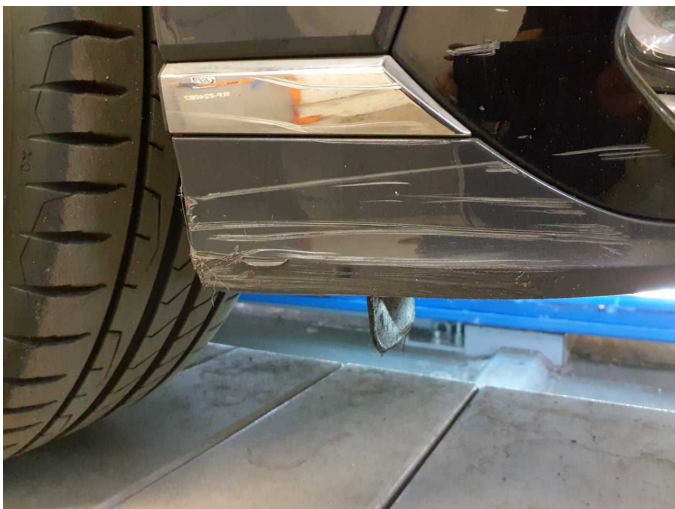
Damage 11: Front bumper: Spoiler (Materialabtrag) - Scratched - Replace
