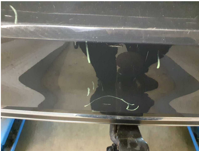
Damage 13: Rear bumper: Rear bumper - Scratched - Paint
