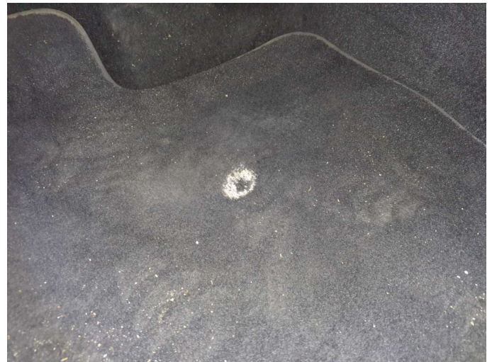
Damage 1: Trim / covers: Floor mats - Holes - Replace
