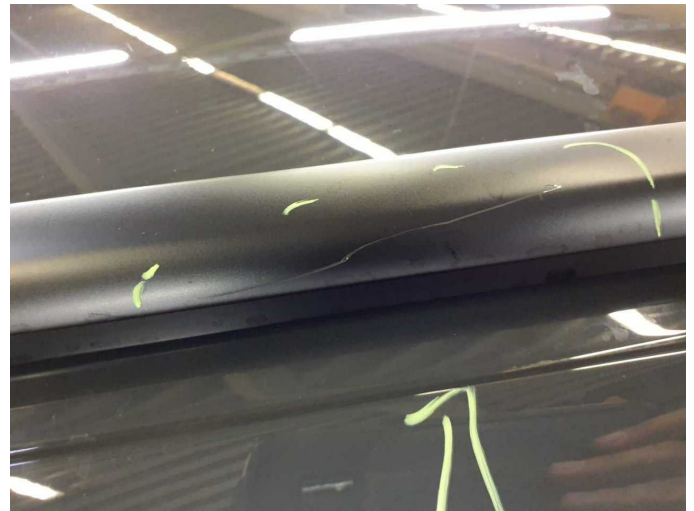
Damage 4: Roof: Roof rail - right side - Scratched - Smart repair
