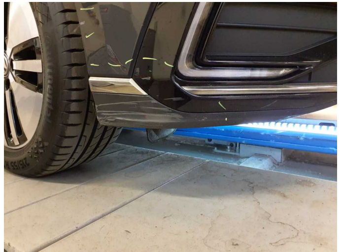
Damage 11: Front bumper: Spoiler (Materialabtrag) - Scratched - Replace
