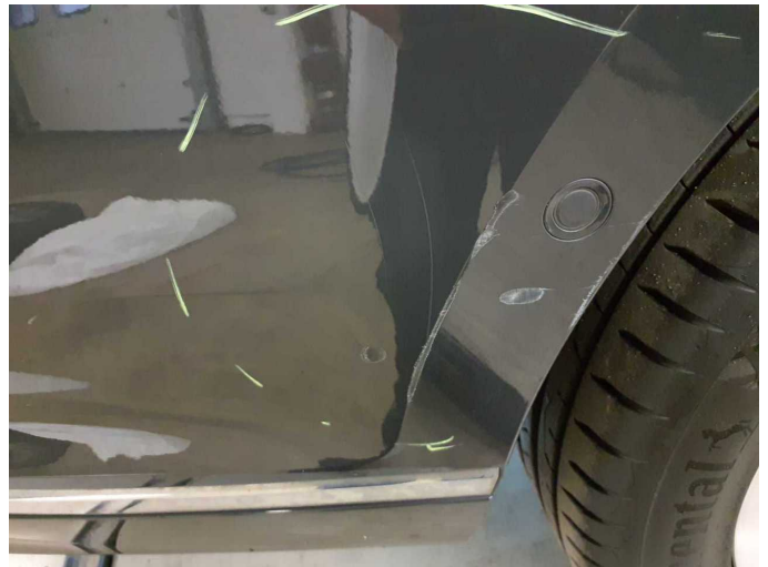
Damage 13: Rear bumper: Rear bumper - Scratched - Paint
