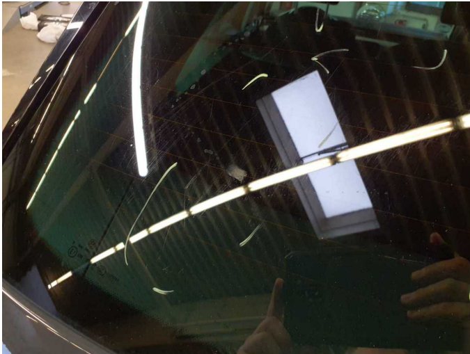
Damage 18: Vehicle glazing: Rear window - Scratched - Replace
