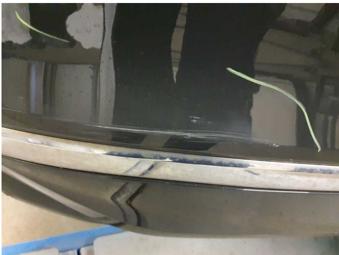
Damage 13: Rear bumper: Rear bumper - Scratched - Paint
