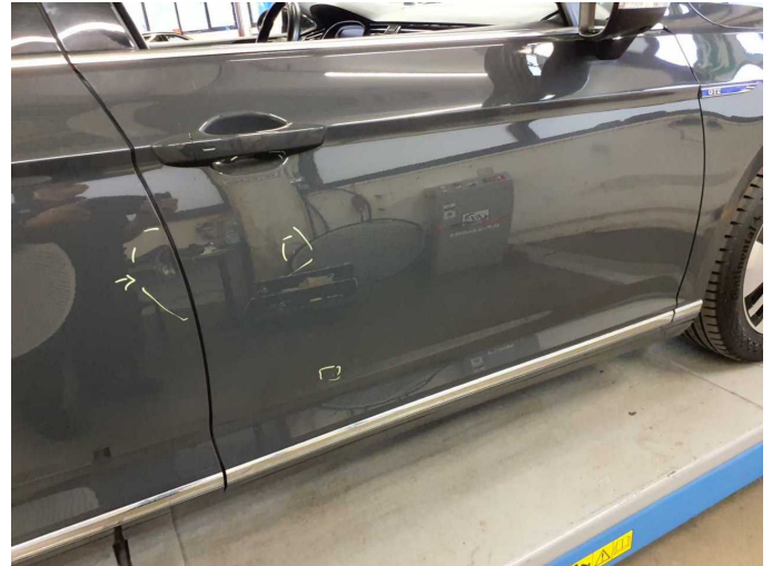
Damage 16: Door - front right side: Door - Scratched - Paint
