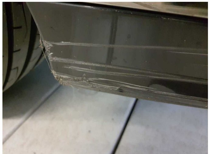
Damage 11: Front bumper: Spoiler (Materialabtrag) - Scratched - Replace
