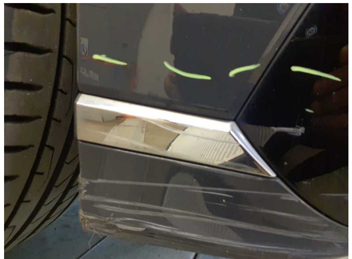
Damage 12: Front bumper: Front bumper - Scratched - Paint
