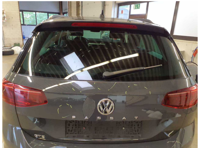
Damage 18: Vehicle glazing: Rear window - Scratched - Replace
