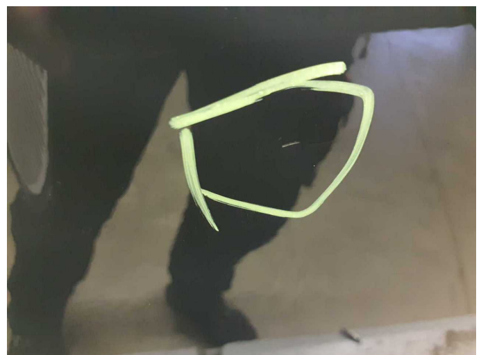
Damage 15: Door - rear left side: Door - Dent / paintcoat damage - Repair and paint
