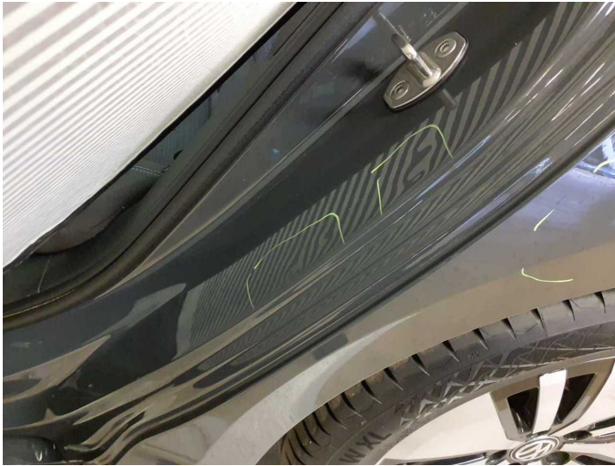
Damage 10: Side panel - rear left side: Sill - dent(s) - Smooth repair work
