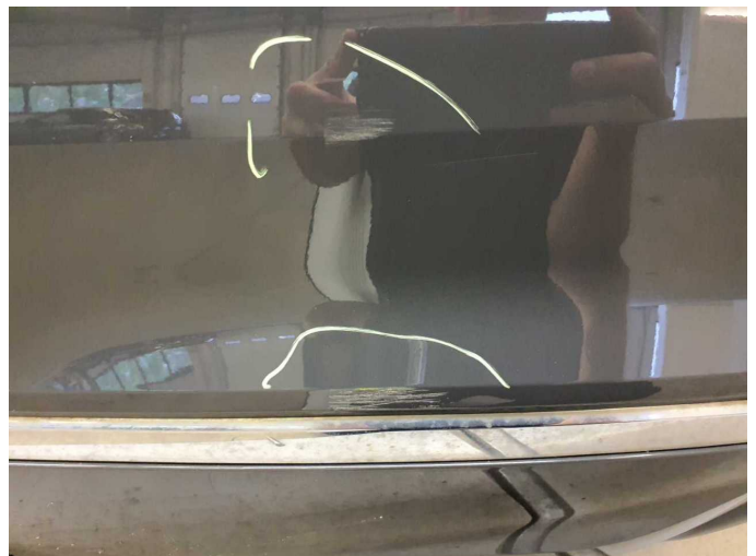
Damage 13: Rear bumper: Rear bumper - Scratched - Paint
