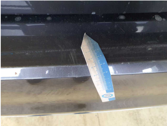
Damage 10: Rear bumper: Rear bumper - Scratch(es) - Paint
