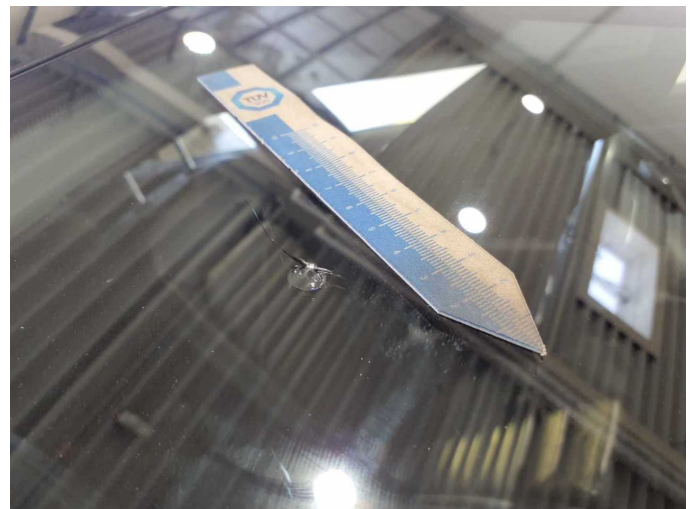
Damage 12: Vehicle glazing: Windscreen - Damaged - Replace
