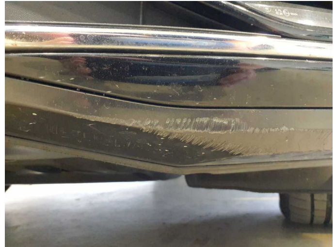
Damage 9: Front bumper: Front bumper - Scratch(es) - Paint
