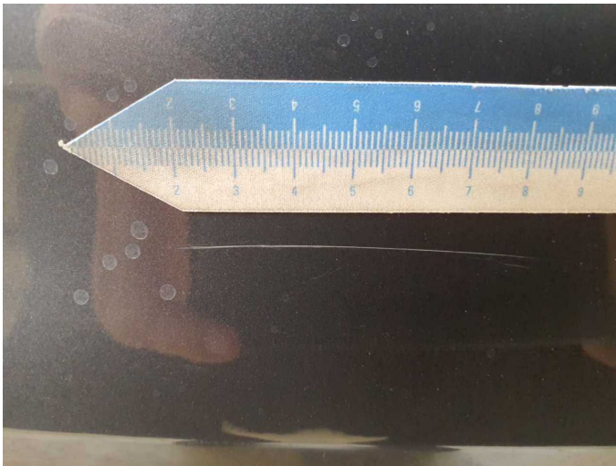
Damage 10: Rear bumper: Rear bumper - Scratch(es) - Paint
