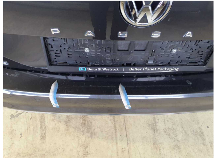
Damage 10: Rear bumper: Rear bumper - Scratch(es) - Paint
