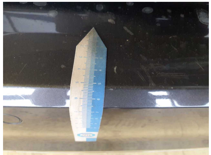
Damage 10: Rear bumper: Rear bumper - Scratch(es) - Paint
