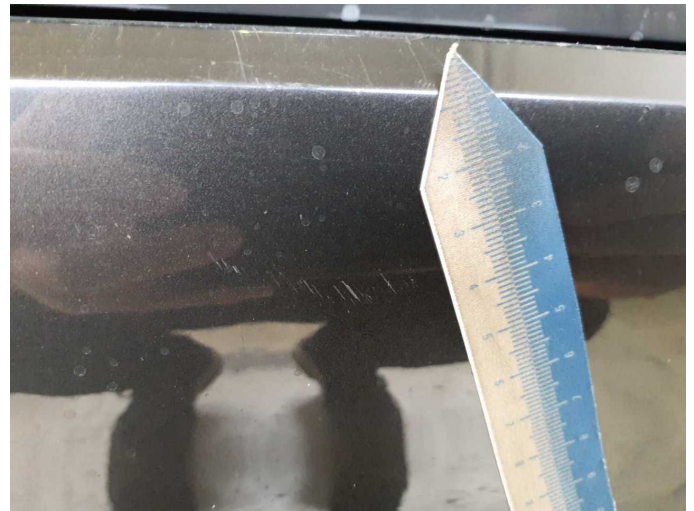
Damage 10: Rear bumper: Rear bumper - Scratch(es) - Paint
