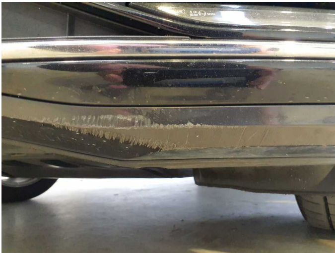
Damage 9: Front bumper: Front bumper - Scratch(es) - Paint
