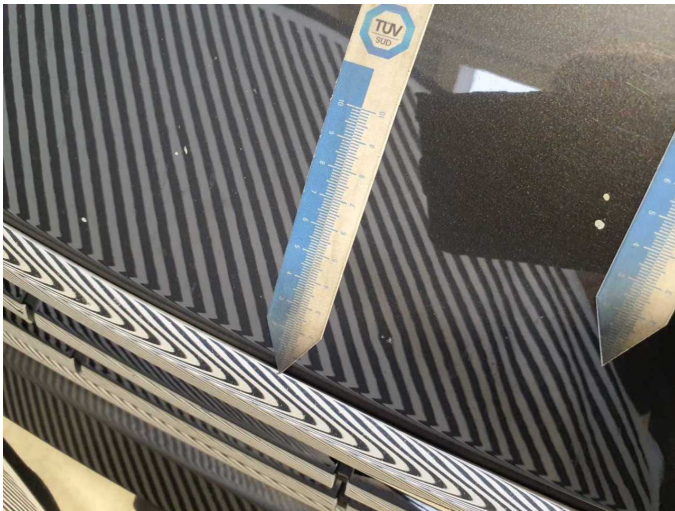
Damage 11: Bonnet: Bonnet - Dent / paintcoat damage - Repair and paint
