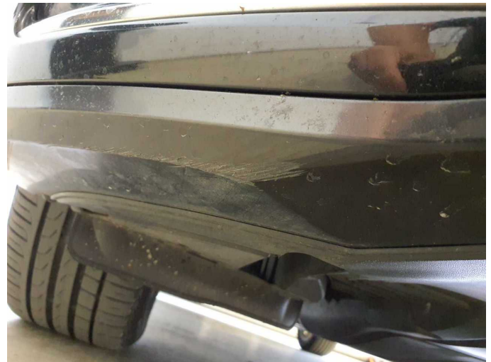
Damage 9: Front bumper: Front bumper - Scratch(es) - Paint
