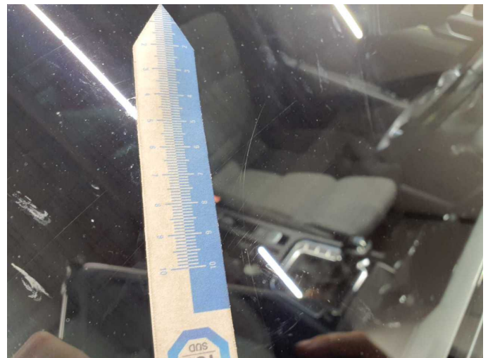
Damage 8: Vehicle glazing: Windscreen - Scratch(es) - Replace
