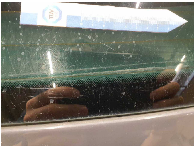
Damage 5: Vehicle glazing: Rear window - Scratched - Replace
