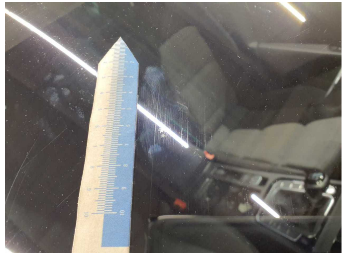
Damage 8: Vehicle glazing: Windscreen - Scratch(es) - Replace
