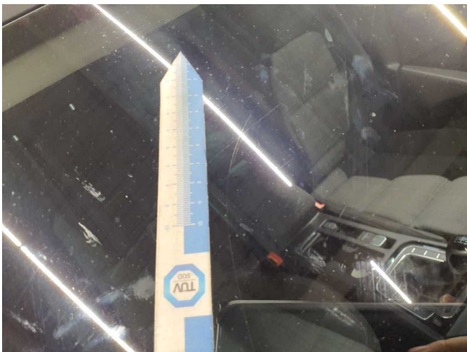
Damage 8: Vehicle glazing: Windscreen - Scratch(es) - Replace
