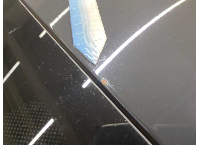
Damage 7: Roof: Roof (Rost) - Stone chips - Paint
