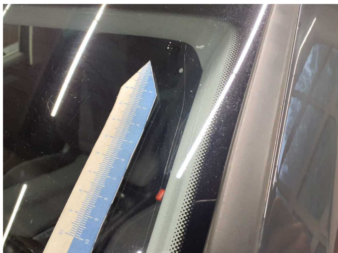
Damage 8: Vehicle glazing: Windscreen - Scratch(es) - Replace
