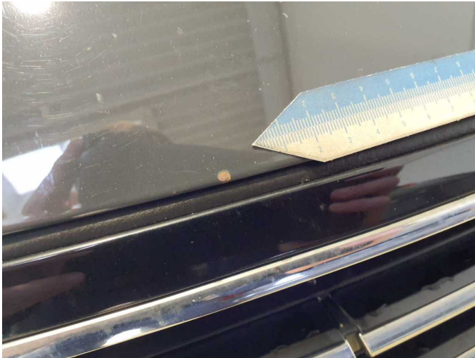
Damage 13: Bonnet: Bonnet - Corrosion - Repair and paint
