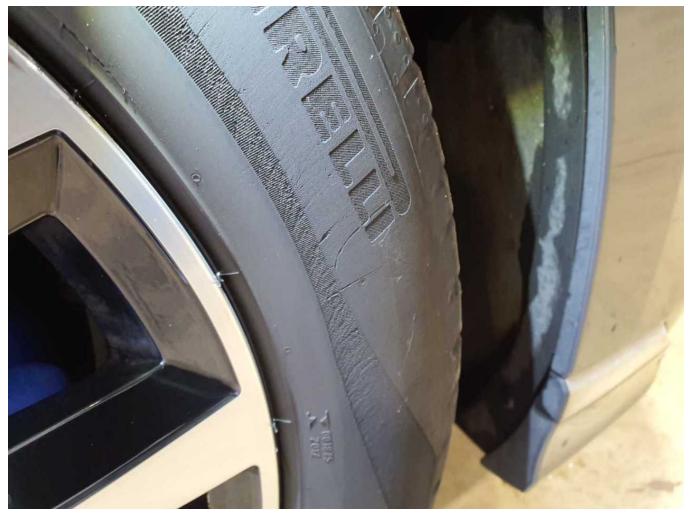
Wear and tear 3: Wheel / tyres: Tyre - front right side - Abrasion - No deduction
