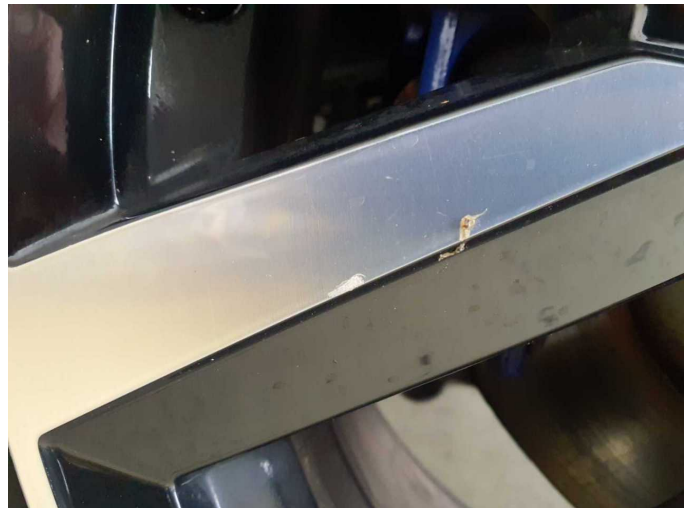
Wear and tear 2: Wheel / tyres: Alloy rim - rear left side - Scratch(es) - No deduction
