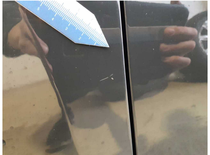
Wear and tear 1: Mudguard - left side: Mudguard - left side - Scratch(es) - No deduction
