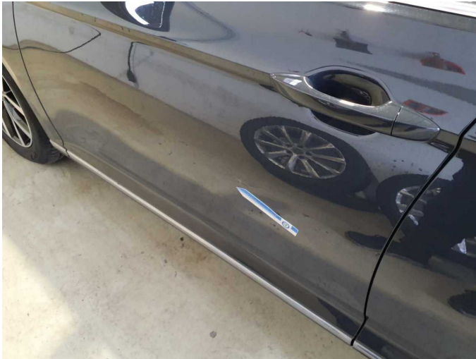
Damage 11: Door - front left side: Door - Scratched - Paint
