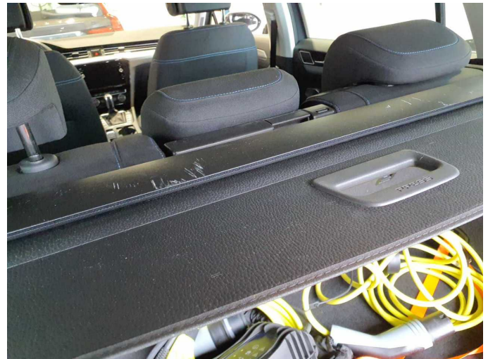
Damage 2: Interior: Boot cover / roller cover - Scratched - Loss in value
