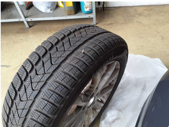
Damage 6: 2nd wheel set: 1 tyre (Fremdkörper) - Damaged - Replace
