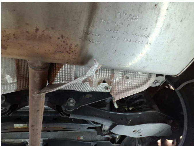
Damage 5: Exhaust system: Heat shield - Broken / torn - Replace
