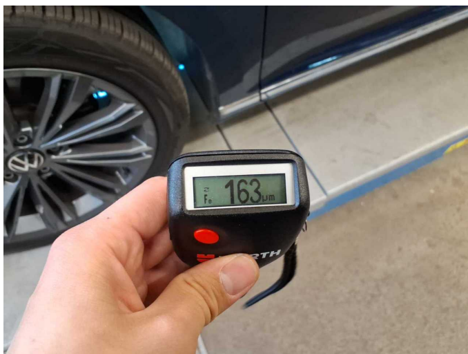
Repainting 1: Roof rail - left side
