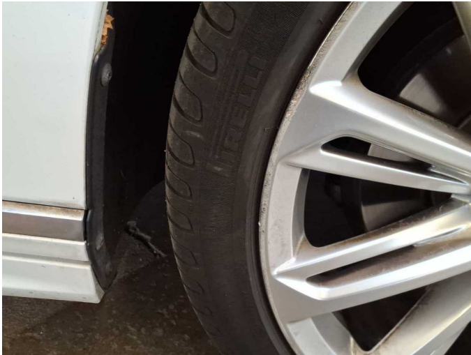
Damage 11: Wheel / tyres: Tyre - front right side (nicht fahrbereit) - Porous / cracked - Replace
