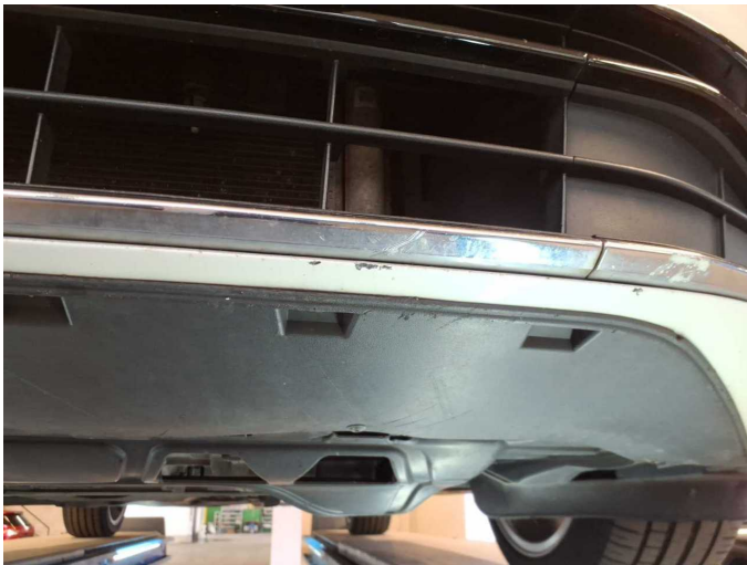
Damage 13: Front bumper: Front bumper - Scratch(es) - Paint
