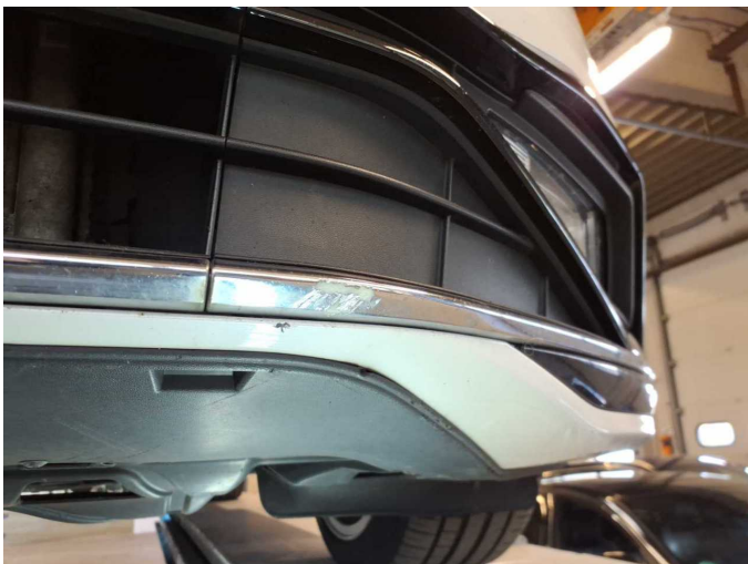
Damage 8: Front bumper: Front bumper (Chromleiste) - Damaged - Replace
