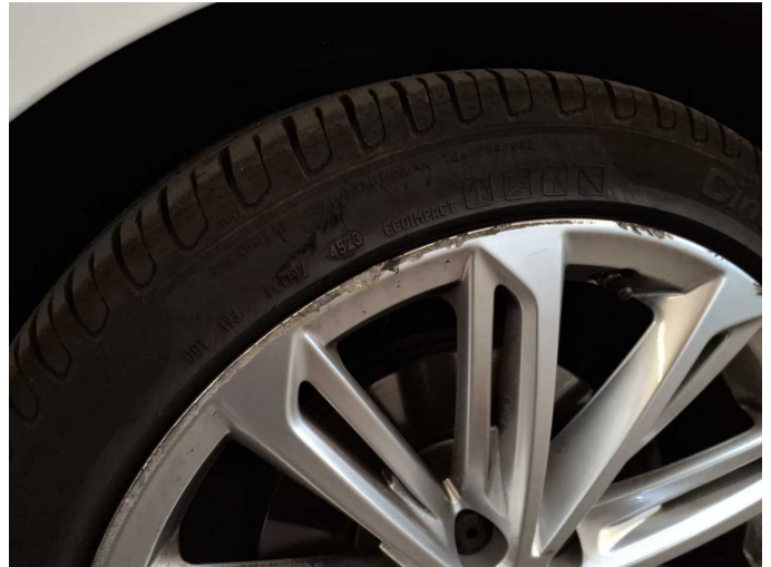
Damage 15: Wheel / tyres: Alloy rim - front right side - Scratched - Replace
