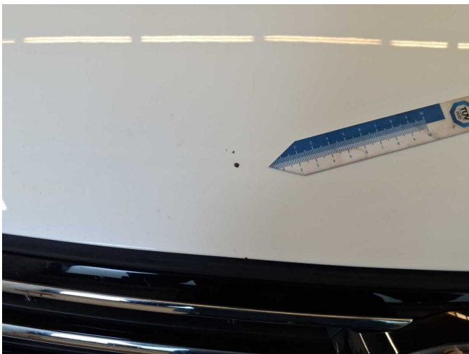
Damage 14: Bonnet: Bonnet - Stone chips - Paint
