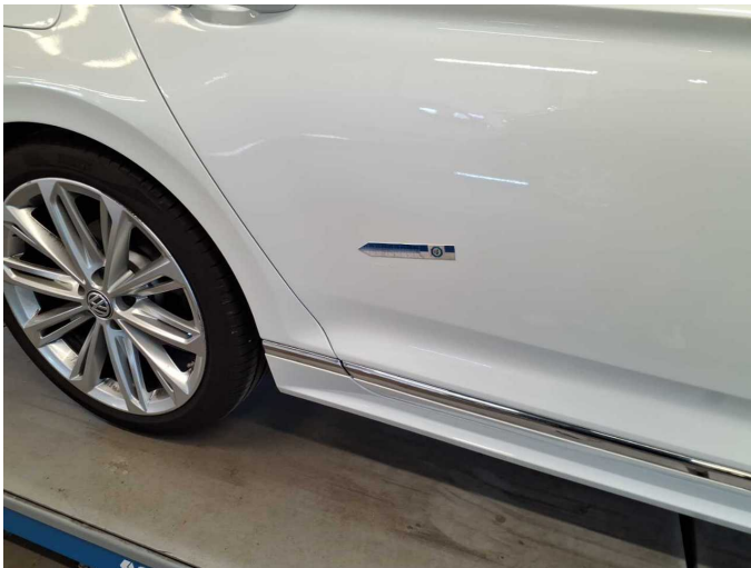
Damage 10: Door - rear right side: Door - Scratch(es) - Smart repair
