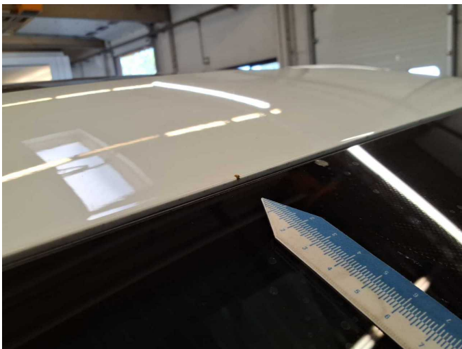
Damage 16: Roof: Roof - Corrosion - Repair and paint
