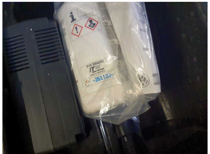
Damage 1: Equipment: Tirefit filler - Expired - Replace
