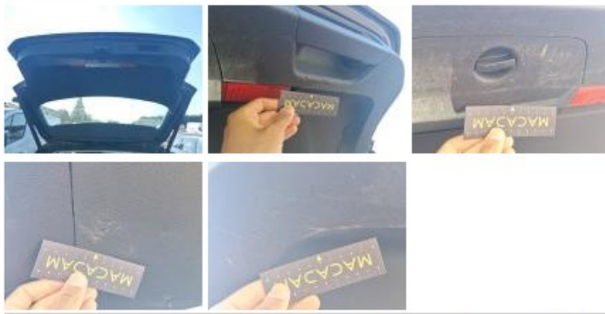
Interior covering C pillar L, Scratch(es), Smart repair
