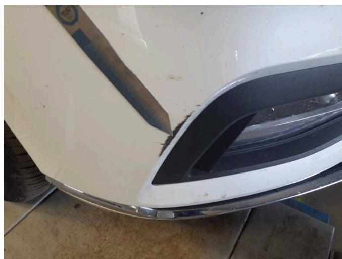
Damage 2: Front bumper: Front bumper - Scratched - Paint
