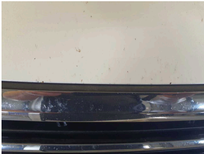
Damage 3: Bonnet: Bonnet - Stone chips - Paint
