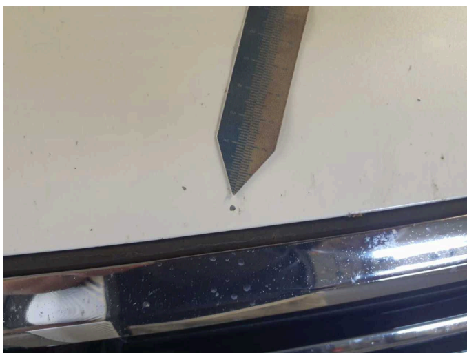
Damage 3: Bonnet: Bonnet - Stone chips - Paint
