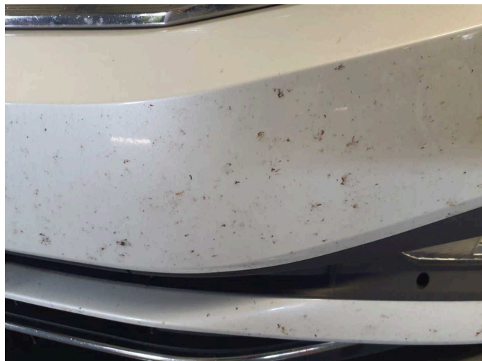
Damage 2: Front bumper: Front bumper - Scratched - Paint
