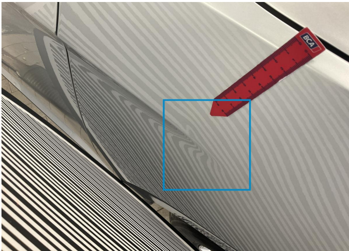
5. Fender / Front Right Bodywork / Dent / Dent -
