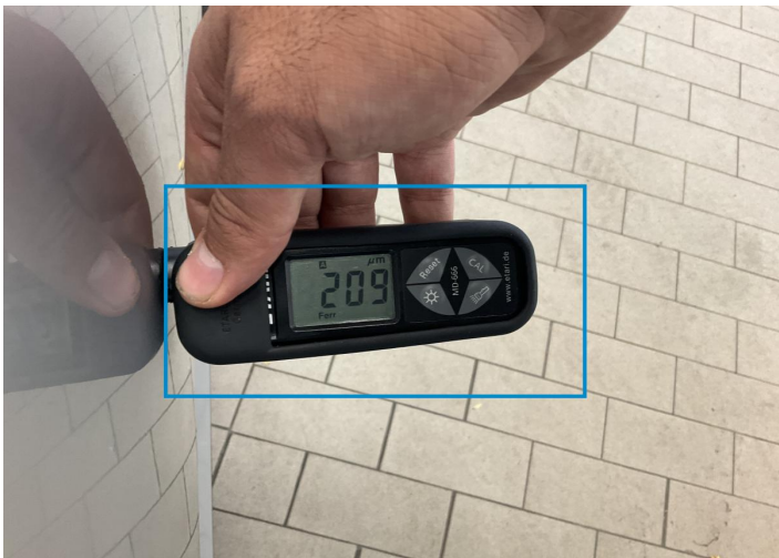
1. Door / Back Left Paint / Poor Previous Repair -
