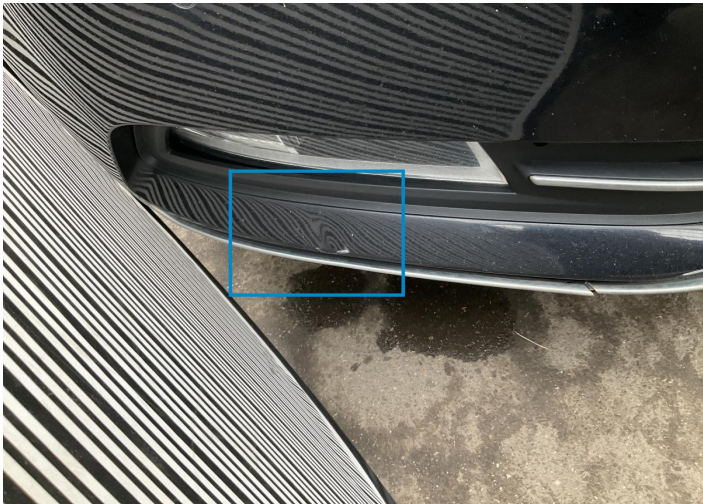
3. Bumper / Front Bodywork / Breakage / Hole -
